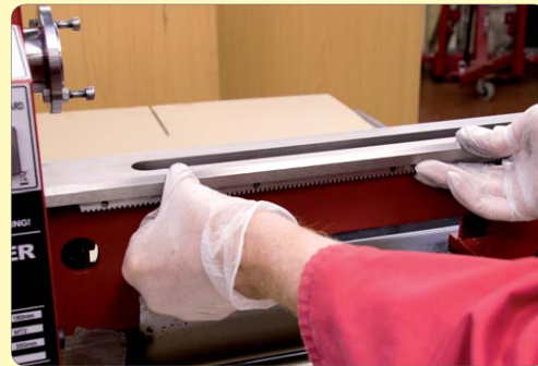
85. Trial fit rack to check if it seats or rocks.
