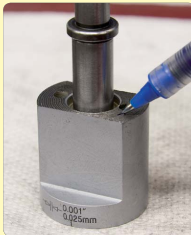
144. To increase backlash, machine a little from the recess. Remove the feed screw and bracket and put to one side.
