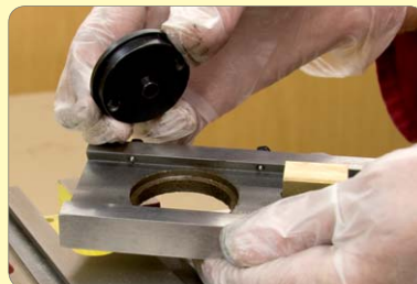
150. Fit top slide base retaining plate.
