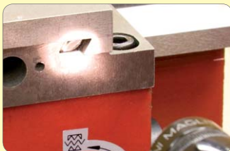
149. View gib strip to check if it's sitting correctly. If OK, disassemble.
