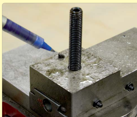
5. Remove the tool post and remove the indexing plunger and spring and keep in a safe place.
