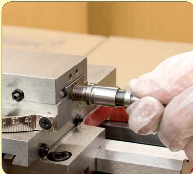
171. Oil / grease feed screw and fit. Oil / grease end of feed screw and bracket and fit.
