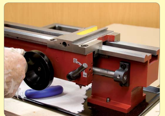
114. Unlock 1/2 nuts and rack saddle up and down bed to check pinion has no tight spots on rack.
