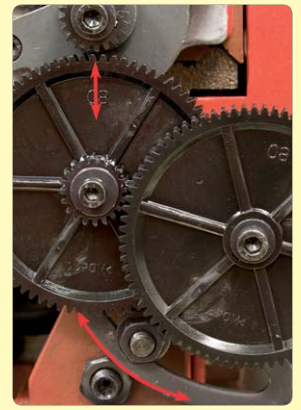
136. Engage quadrant and adjust backlash between gears A and B.
