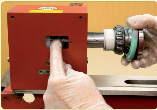
65. Assemble spindle aligning keyways in spacer, speed encoder and gears.
