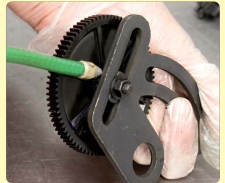
125. Oil the lower quadrant gear shaft.
