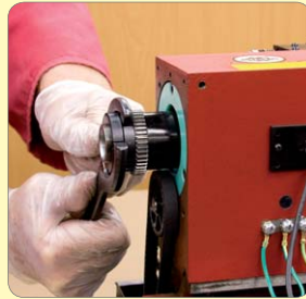
81. Adjust the bearings for "slight drag" and pinch up the C nuts for the moment. Following the Start Up Procedure on page 18, run the spindle to warm it up and settle the grease. Check and adjust the preload again. Lock the C nuts when the preload appears to be OK. Take care not to overdo the preload as this could overheat and damage the bearings.
