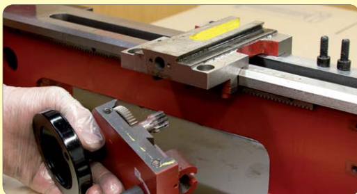
28. Undo the screws securing the apron and remove.
