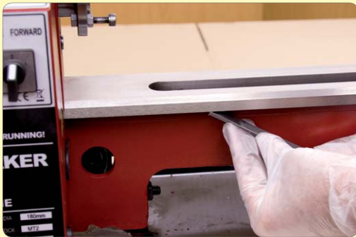
84. Scrape any point off the bed shears.
