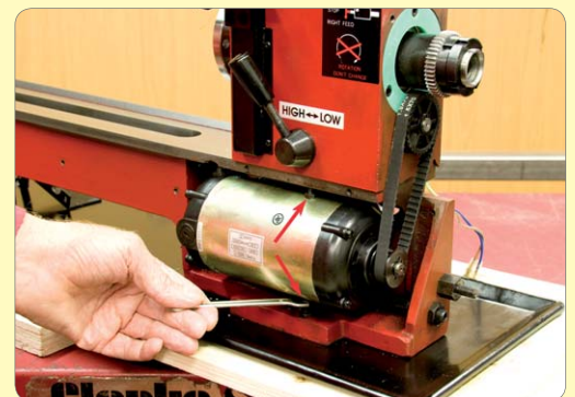
40. Slacken the two drive belt adjusting screws.
