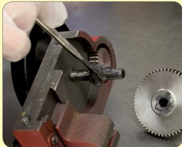
103. Grease or oil pinion gear and shaft assembly
