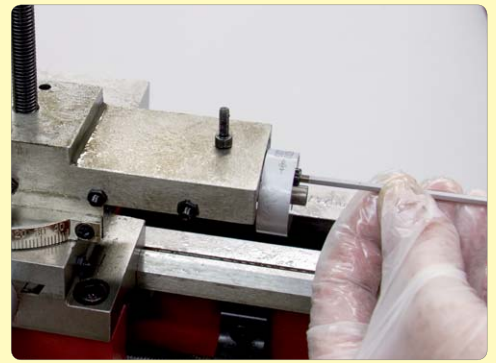
8. Remove the leadscrew end plate.
