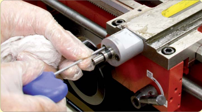
17. Remove the leadscrew end plate and leadscrew.
