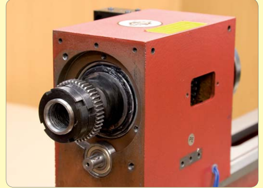
70. Lubricate threads and fit C nuts - hand tight only.
