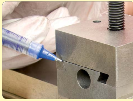
167. Temporarily fit top slide to compound base and check for clearance in corners of dovetail.
