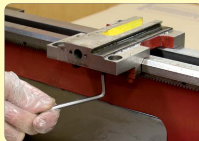
29. Slacken the saddle adjusting screws and slide the saddle off the end of the bed.
