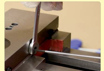
163. Make final adjustments to the gib screws for free movement of the handle with little drag.
