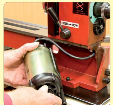
42. Undo the motor mount pivot screws enough to remove the motor.
