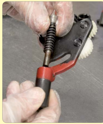
122. Strip, clean, oil / grease and reassemble the tumbler reverse detent assembly.
