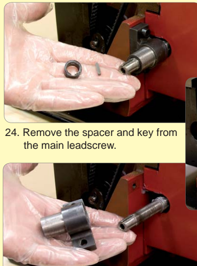
25. Remove the leadscrew carrier bracket.
