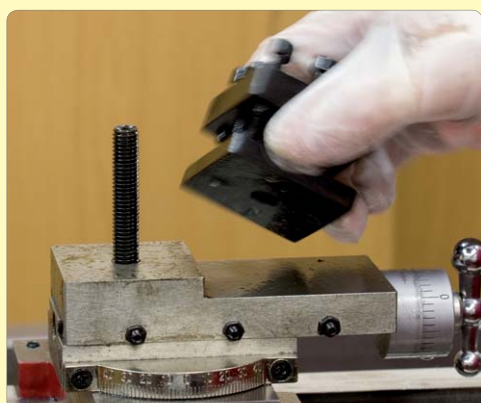
5. Remove the tool post and remove the indexing plunger and spring and keep in a safe place.
