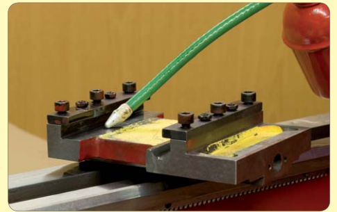
93. Oil bed and saddle and slide saddle onto bed.
