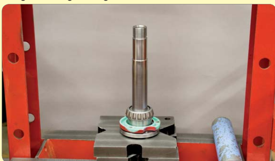
61. The new bearing in place.
