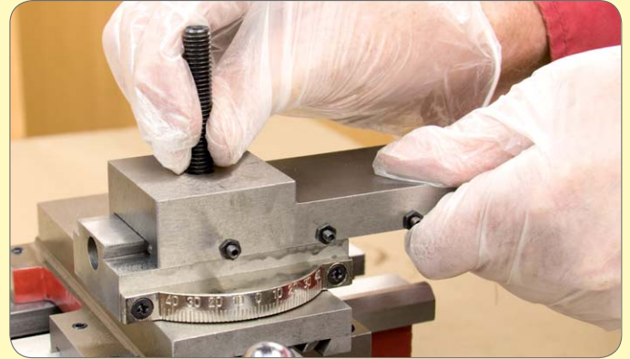
170. Adjust the screws so the slide will move back and forth easily by hand.
