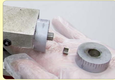
7. Tap compound slide along with a soft mallet to remove micrometer dial and friction clip.
