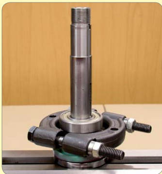
53. Press or pull off bearing and remove bearing cover from spindle. If the bearing is tight to remove, polish the spindle to make the bearing a Push Fit otherwise you will not be able to preload the taper roller bearings accurately.
