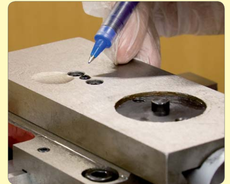
159. The centre screw is for adjusting the position of the nut in an up/down direction and the two outside screws are for locking. Slacken all three screws for now.
