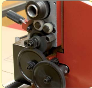
138. Run spindle to check for noisy gear meshing and readjust backlash if necessary.
