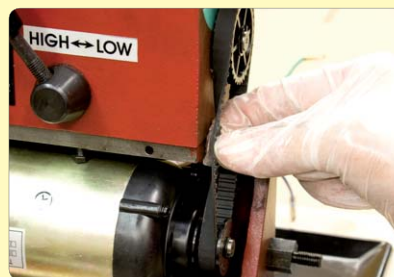
75. Refit the drive belt and adjust tension. If you cannot twist the belt through 90° quite easily, the tension is probably too tight.
