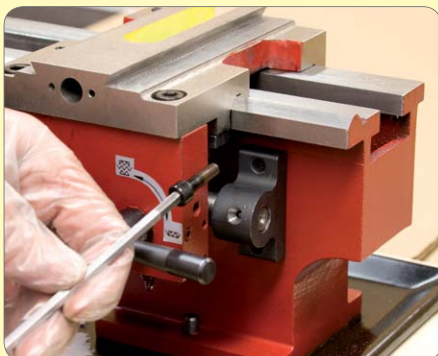
115. Return saddle close to leadscrew bracket and lock 1/2 nuts. Remove bracket screws.
