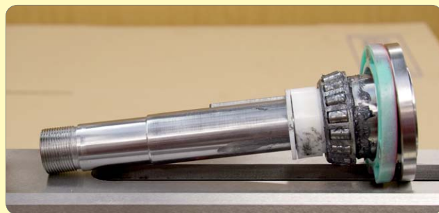
64. Refit the key, the original spacer + the small 0.110" (2.8mm) thick spacer (the original small spacer reduced in thickness) to the spindle and grease the bearing.
