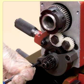
127. Grease the gear shaft and fix the gear carrier to the cover.
