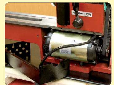
76. Thread mains cable through but do not fit motor cover yet.
