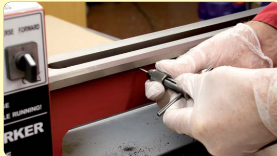
87. Drill and tap the fixing holes deeper if necessary.
