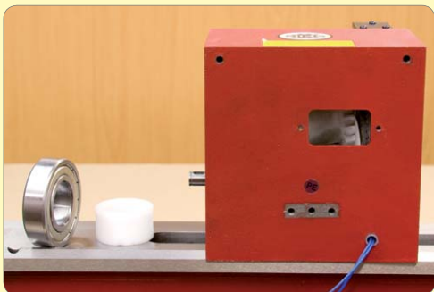
55. Press or drift-out rear bearing and remove the large white plastic spacer.
