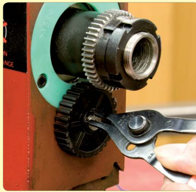
44. Remove circlip & pull off drive pulley.
