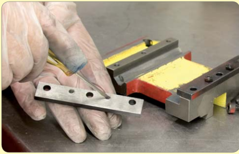
92. Loosen shear plate adjusting screws below the level of the plate and loosely fit to saddle.
