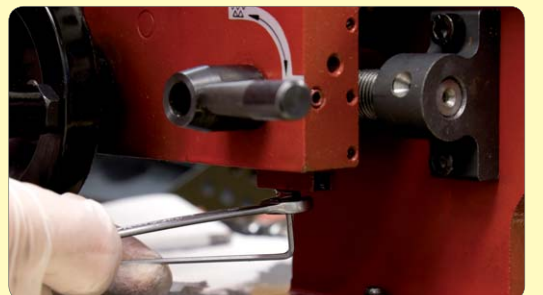
120. Check bite of 1/2 nuts on leadscrew is not too tight. Slacken 1/2 nut adjusting screw. Lock 1/2 nuts. Screw in adjusting screw until it touches and then a further 1/8th turn. Lock off.
