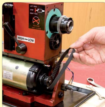
41. Slacken the motor mount pivot screws and remove the drive belt.
