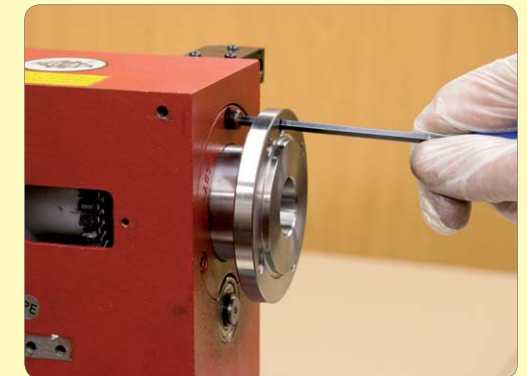
73. Secure front bearing cover.
