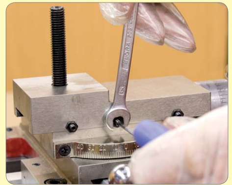
177. Final adjust the top slide gib to your preference and lock-off the screws.
