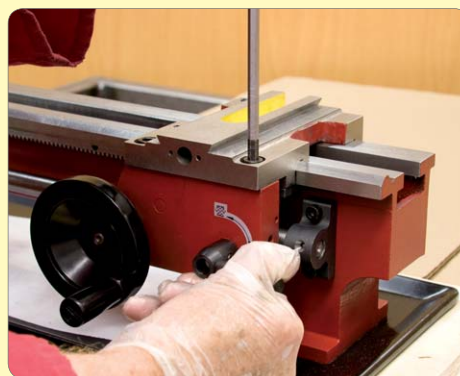
113. Lock 1/2 nuts onto leadscrew and tighten apron fixing screws.
