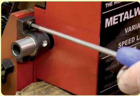
109. Loosely fit leadscrew bracket & grease bore.
