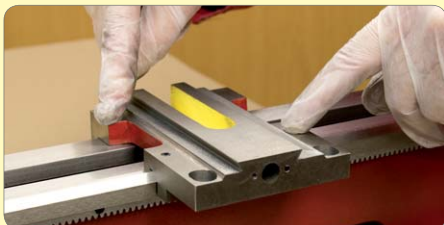
87. Drill and tap the fixing holes deeper if necessary.
