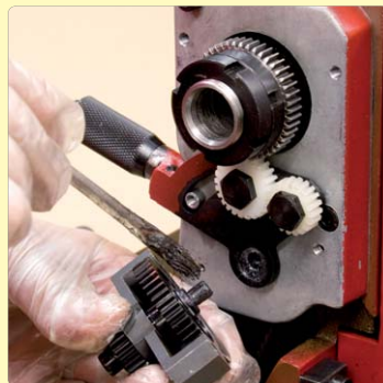
127. Grease the gear shaft and fix the gear carrier to the cover.
