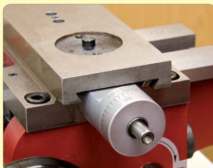
164. Remove the handle again in order to fit the micrometer dial and friction spring.
