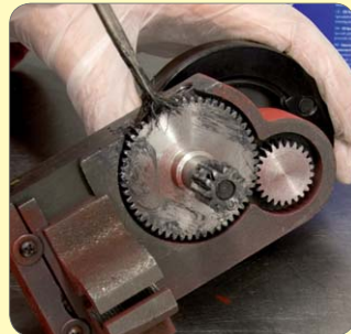
101. Check there is no rock on the 1/2 nuts.
