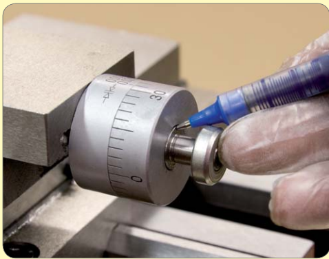
176. Backlash can often be reduced by turning a recess in the spacer to clear the shoulder on the end of the feed screw. The recess depth should be slightly less than the measurement taken with the feeler gauge to allow some clearance. Adjust for free movement with minimal backlash.
