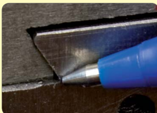
145. Place cross slide on saddle and check for clearance in corners of dovetail.
