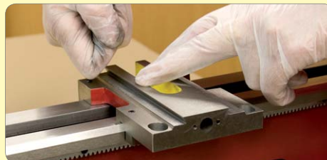
87. Drill and tap the fixing holes deeper if necessary.
