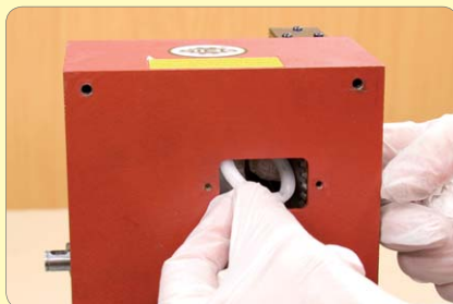
56. Remove the small white plastic spacer through the speed display pickup hole. Reduce the thickness of this spacer to 0.110" (2.8mm) before refitting later.
