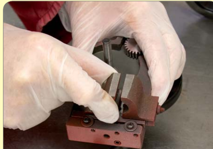
101. Check there is no rock on the 1/2 nuts.
