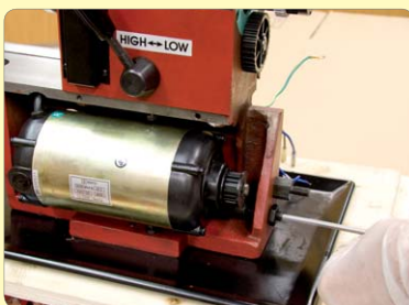
74. Refit the motor onto it's pivot screws.
