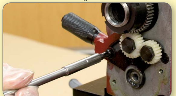
22. Undo and remove the tumbler reverse arm.
