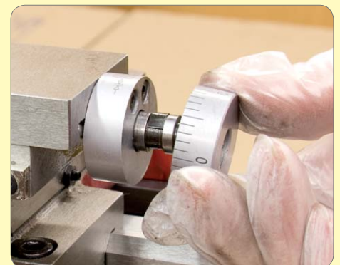
173. Assemble and fit the micrometer dial and friction clip to feed screw.
