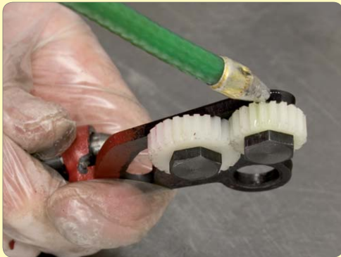
123. Oil the tumbler reverse gear shafts.
