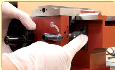
119. Return saddle to tailstock end and lock 1/2 nuts. Rock handwheel back and forth with finger over end of leadscrew to check for end float. Tap brackets in to remove end float.
