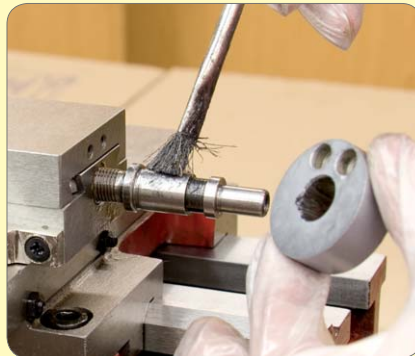
171. Oil / grease feed screw and fit. Oil / grease end of feed screw and bracket and fit.
