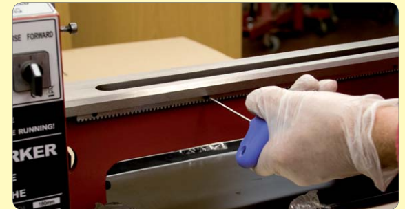
88. Final fit rack making sure it seats properly in the corner.
