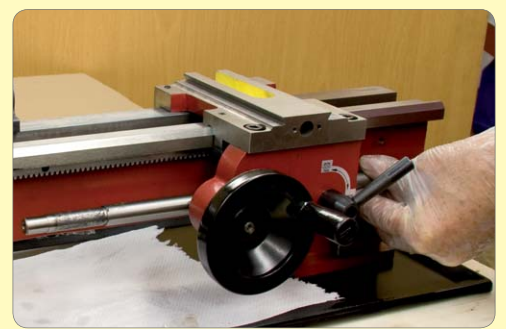
110. Grease end of leadscrew and feed through 1/2 nut and into bracket at headstock end.
