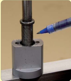
154. Grease / oil the feed screw and bracket.
