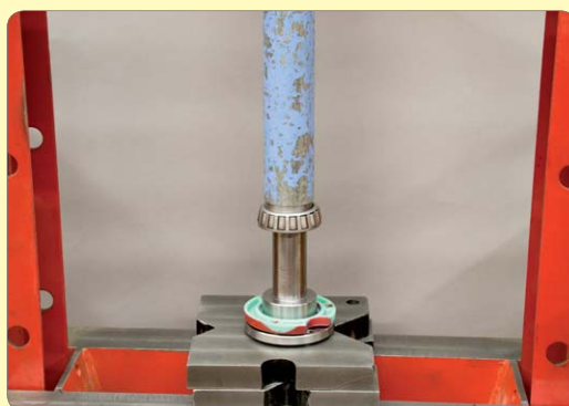
60. Refit front bearing cover to spindle and press on new 30206 taper roller bearing inner
