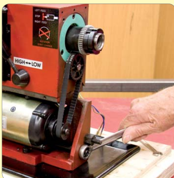
41. Slacken the motor mount pivot screws and remove the drive belt.
