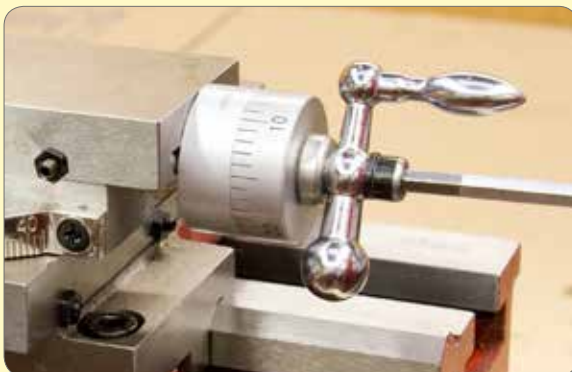
170. Fit the spacer and handle and wind the slide back and forth.
