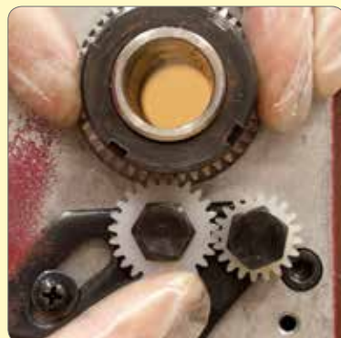
118. Check free play in gears: Forward...
