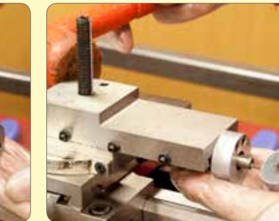
15. Tap the compound slide to remove the micrometer dial taking care not to lose the friction spring.
