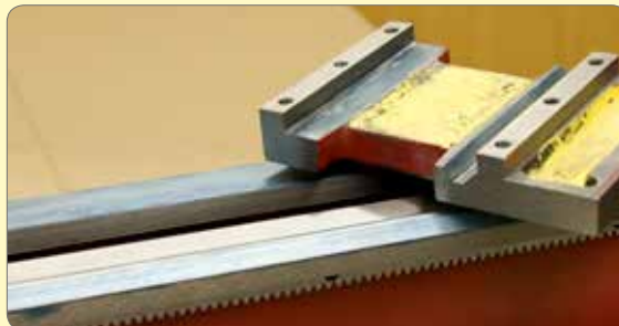
88. Place the saddle on the bed and check to see how it sits.
