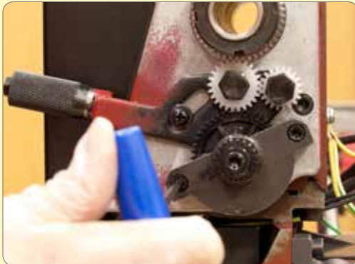
122. Fit the transfer gear assembly.
