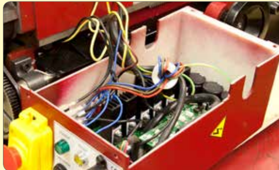
36. Remove 4 screws retaining the control panel and lay it down beside the machine.
