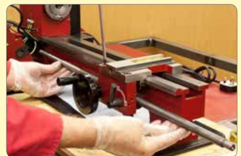
105. Grease end of leadscrew and feed through 1/2 nut and into bracket at headstock end.
