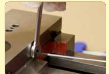
159. Make final adjustments to the gib screws for free movement of the handle with little drag.
