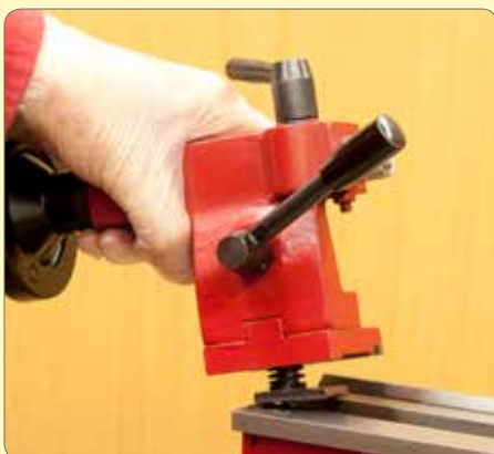
5. Remove the tailstock.
