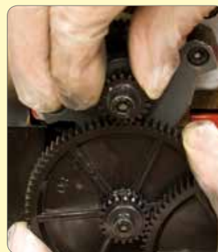
129. Engage quadrant and adjust backlash between gears A and B.
