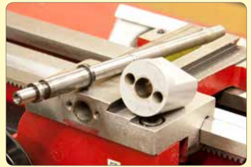
25. Remove the cross slide feed screw.
