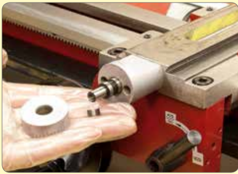
23. Remove the micrometer dial & friction spring.
