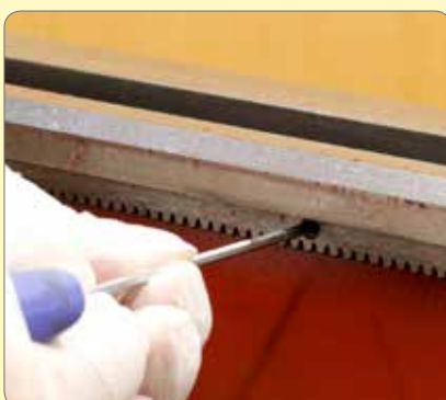
31. Remove the screws holding the rack.
