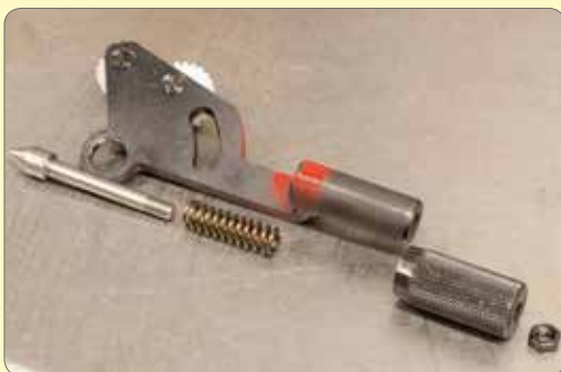
115. Strip, clean, oil / grease and reassemble the tumbler reverse detent assembly.
