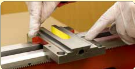
86. Drill and tap the fixing holes deeper if necessary.
