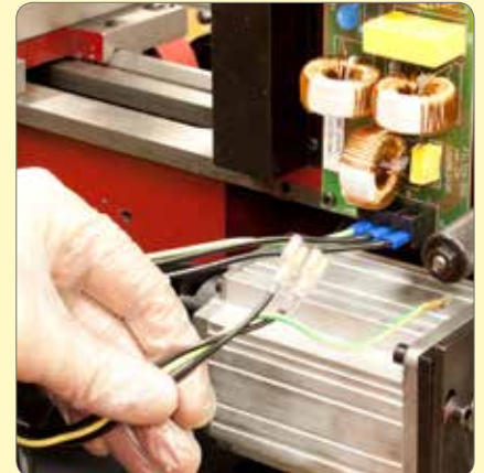
39. Remove the motor cover and pull power cables through from front of machine.
