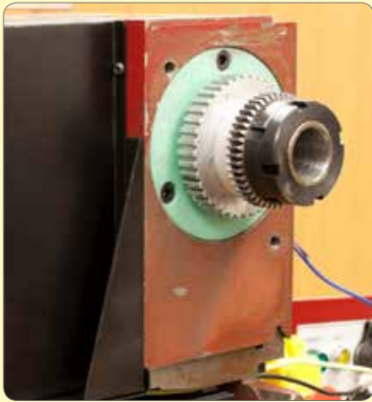
76. Remove the tumbler reverse assembly and belt cover again.
