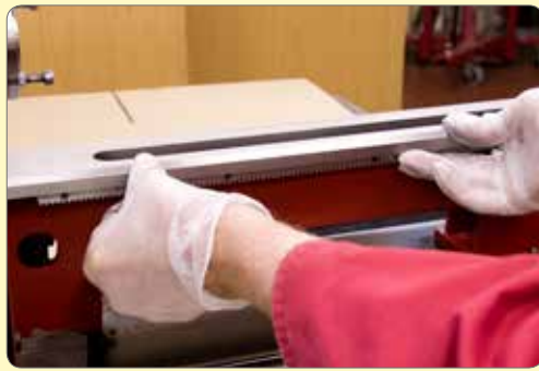
84. Trial fit the rack to check if it seats well or rocks.
