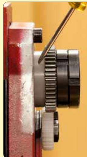
75. Adjust this spacer to correctly align the two gears.
