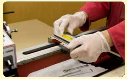
98. Test slide saddle up and down the bed. There should be slight drag with no free play. Lightly pinch up remaining cap screws checking after each one and adjusting as required.
