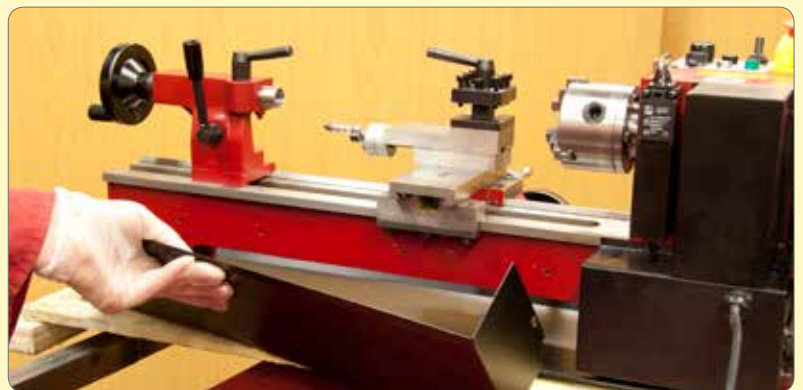
4. Remove the rear splash guard..
