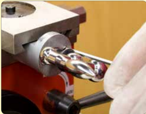
153. Slacken the bracket screws, wind the slide right back and tighten the screws.
