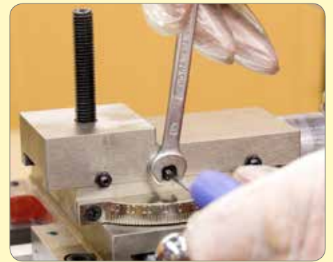
173. Final adjust the top slide gib to your preference and lock-off the screws.
