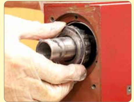
59. Grease the rear race and rollers and fit.
