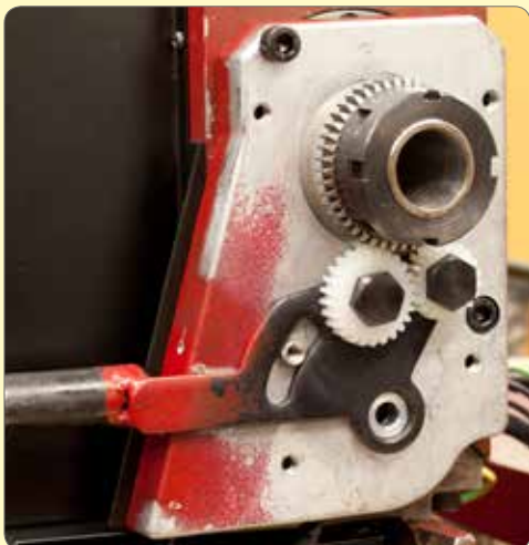
73. Temporarily fit the belt cover and tumbler reverse lever assembly.
