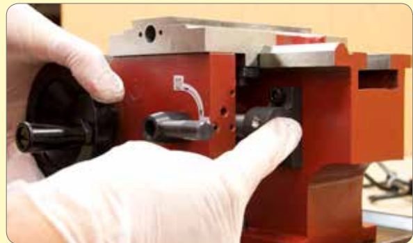
114. Return saddle to tailstock end and lock 1/2 nut. Rock handwheel back and forth with finger over end of leadscrew to check for end float. Tap brackets in to remove end float.
