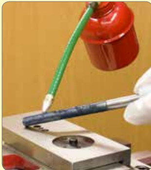
149. Fit adjusting screws and adjust so slide can be moved back and forth easily by hand.
