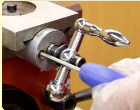
153. Slacken the bracket screws, wind the slide right back and tighten the screws.
