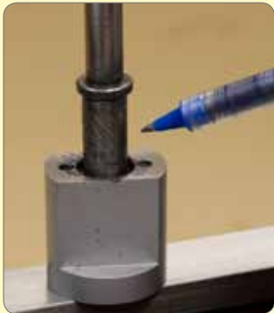
150. Grease / oil the feed screw and bracket.
