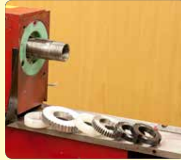
46. Remove lock nuts, gear, belt pulley, 2 spacers and the key from the spindle rear.
