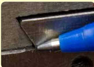
141. Place cross slide on saddle and check for clearance in corners of dovetail.
