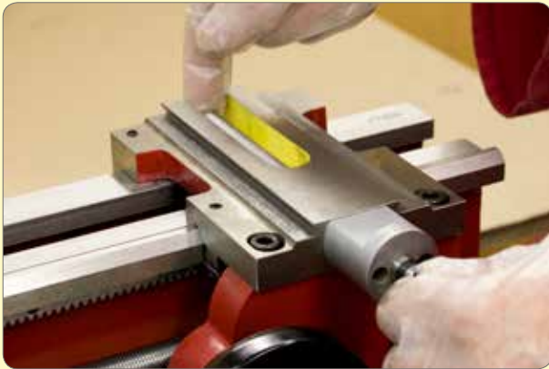
138. Temporarily fit the cross slide feed screw and bracket and check for backlash.
