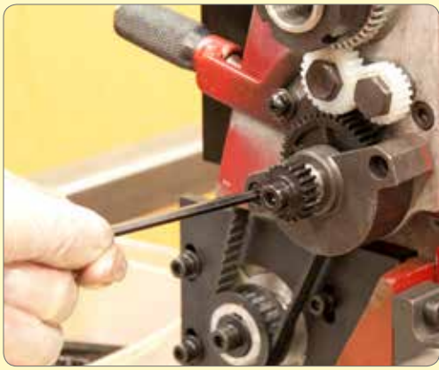
8. Remove the transfer gear bracket.
