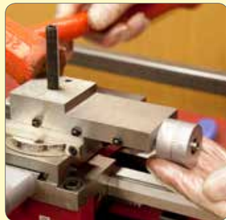
15. Tap the compound slide to remove the micrometer dial taking care not to lose the friction spring.
