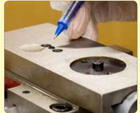
155. The centre screw is for adjusting the position of the nut in an up/down direction and the two outside screws are for locking. Slacken all three screws for now.
