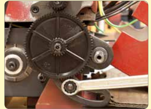
124. Temporarily fit the gear quadrant. DO NOT engage the gears.
