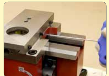
144. Fit adjusting screws lightly.
