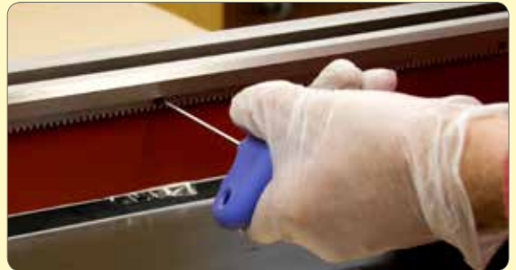
87. Final fit rack making sure it seats properly in the corner.
