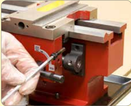
110. Return saddle close to leadscrew bracket and lock 1/2 nut. Remove bracket screws.
