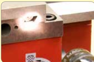
145. View gib strip to check if it's sitting correctly. If OK, disassemble.
