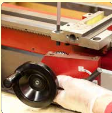
29. Undo two screws to remove the apron from the saddle.
