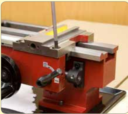
107. Slightly loosen apron fixing screws.
