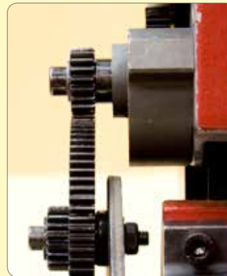
126. "Tweak" the lower quadrant bracket until the gears are in proper alignment.
