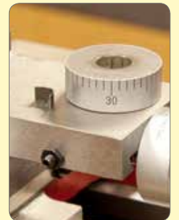
15. Tap the compound slide to remove the micrometer dial taking care not to lose the friction spring.
