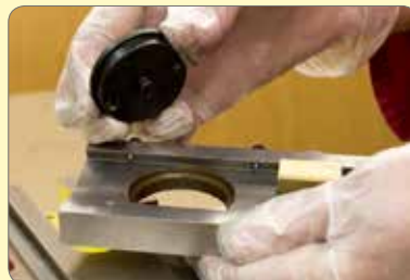
146. Fit top slide base retaining plate.
