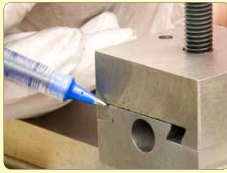
163. Temporarily fit top slide to compound base and check for clearance in corners of dovetail.
