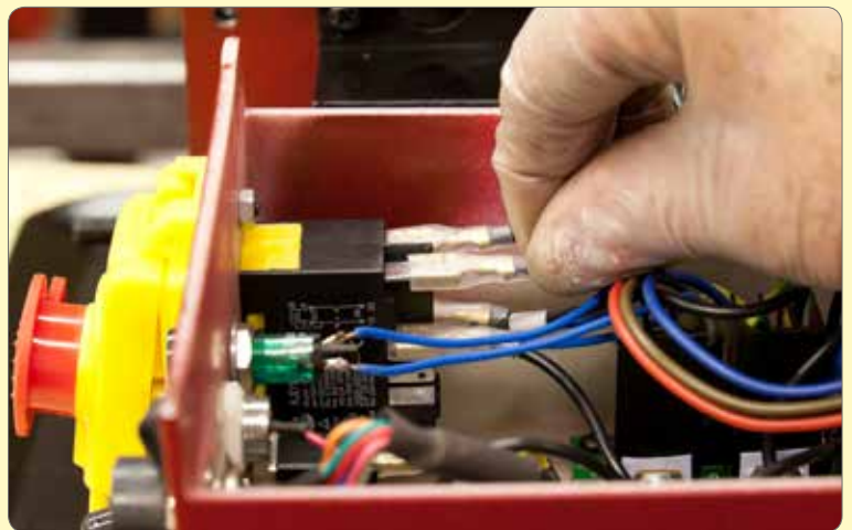
72. Fit the power wires to the emergency stop switch (noting correct orientation) and fit the guard switch wires.
