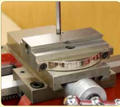
162. Fit compound base to cross slide.
