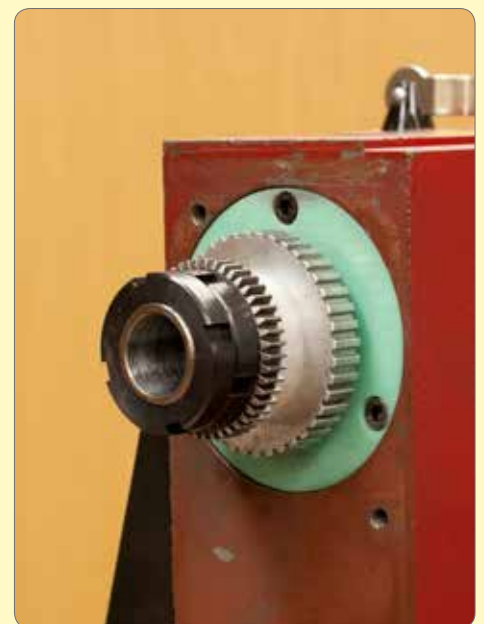
65. Fit the spindle C nuts, adjust out bearing backlash with minimum preload and only nip up the C nuts for the time being.
