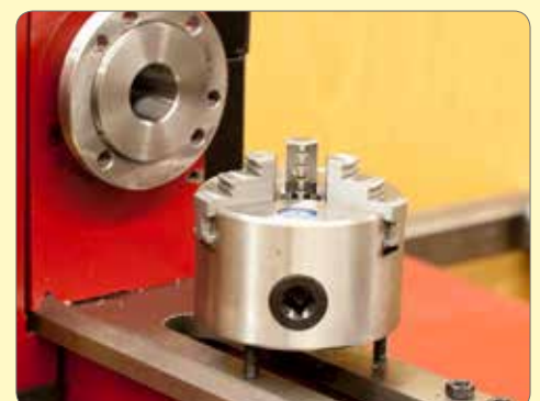
33. Remove the chuck from the spindle flange.
