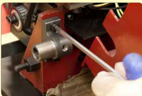
104. Loosely fit leadscrew bracket & grease bore.
