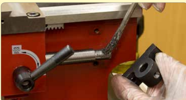
106. Grease end of leadscrew and bracket bore and temporarily fix in place.
