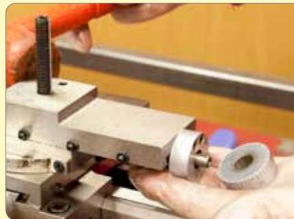
15. Tap the compound slide to remove the micrometer dial taking care not to lose the friction spring.
