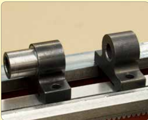
101. The leadscrew brackets as they come on the machine. Notice there is no means of lubricating the bearing surfaces other than at each end of the bracket.
