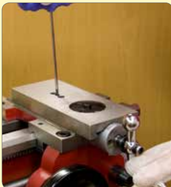
154. Wind the cross slide in and out. If there is any tightness, the feed screw nut will need adjusting.
