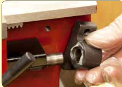
26. Remove left hand and right hand lead screw carrier brackets.
