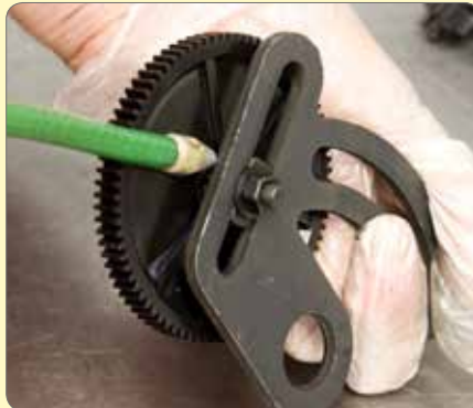
123. Oil the lower quadrant gear shaft.
