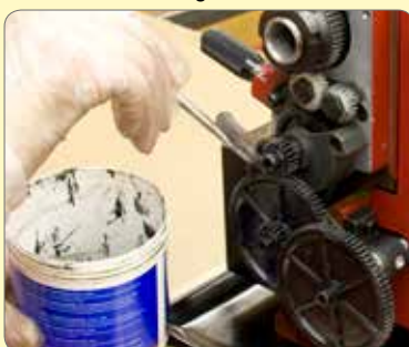
130. Very lightly grease gears.
