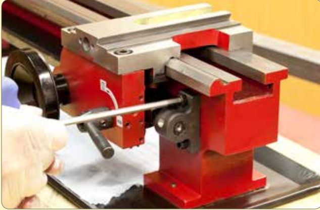
136. Fit the leadscrew bracket with the 1/2 nut locked for position.
