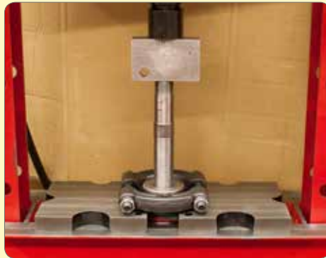
49. Press out the rear bearing.
