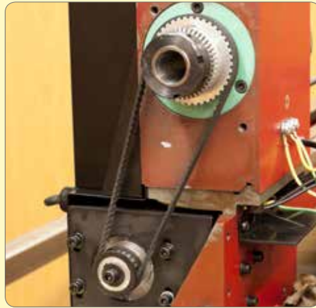
77. Fit the drive belt and adjust the belt tension.
