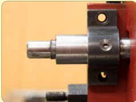
113. Check the bracket holes align with holes in bed. If the holes are misaligned, slot the bracket holes to correct and refix the screws.
