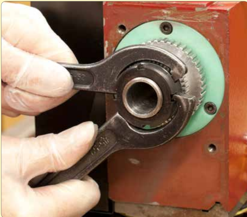
81. After running the spindle to warm it up and settle the grease, check and adjust the preload again. Lock the C nuts when the preload appears to be OK. Take care not to overdo the preload as this could overheat and damage the bearings.
