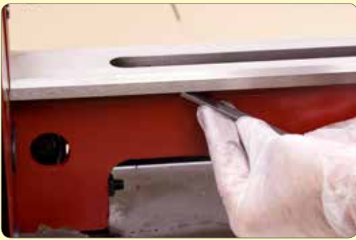
83. Scrape any paint off the bed shears.
