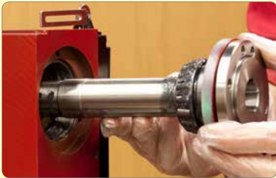
57. Grease the front race and rollers and assemble.
