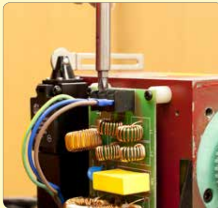
69. Connect Mains In to top of board.
