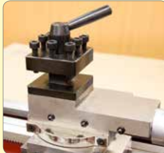
174. Grease and fit the tool post spring and plunger and fit the tool post.
