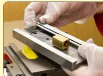
147. Drop in gib strip and lubricate all ways.
