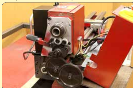
128. Adjust backlash between gears C and D.
