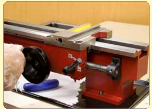
109. Unlock 1/2 nut and rack saddle up and down bed to check pinion has no tight spots on rack.
