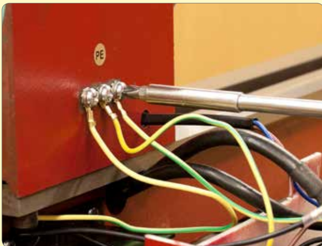
71. Reconnect the earth wires to the head.
