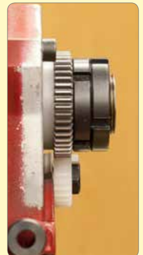
75. Adjust this spacer to correctly align the two gears.
