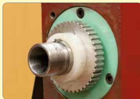
61. Fit the key and plastic spacer.
