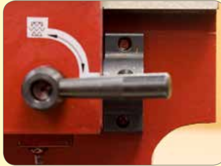
111. Check the bracket holes align with the holes in bed. If holes are misaligned, slot the bracket holes to correct and refix screws.
