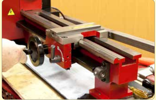
137. Wind the carriage up and down the bed to check guard clears and tighten the screws.
