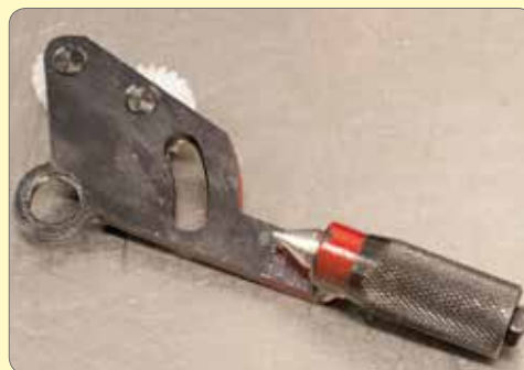
115. Strip, clean, oil / grease and reassemble the tumbler reverse detent assembly.
