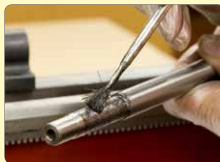
105. Grease end of leadscrew and feed through 1/2 nut and into bracket at headstock end.
