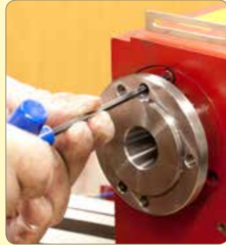
45. Remove the front bearing cover screws.
