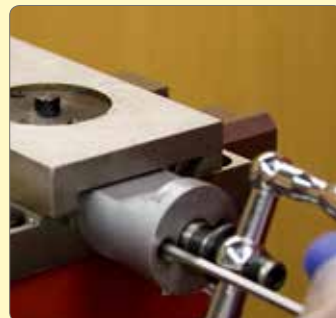
159. Make final adjustments to the gib screws for free movement of the handle with little drag.
