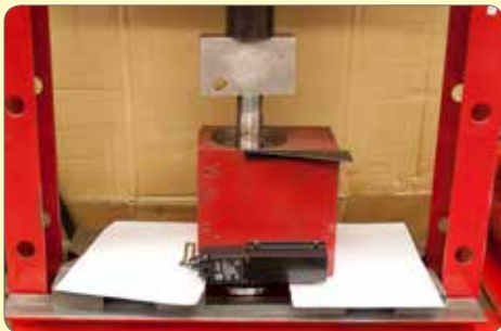
48. Press out the spindle assembly.
