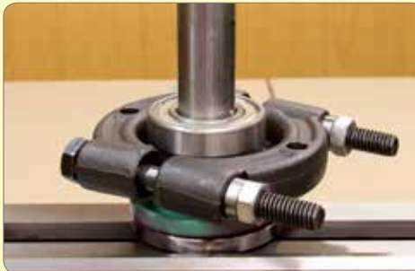
51. Press or pull off bearing and remove bearing cover from spindle. Note the bearing fit. If the bearings are tight to remove, polish the spindle journals. The front bearing can be a press fit on the shaft but the rear bearing needs to be push fit to allow accurate preload adjustments to be made by the two C-nuts.
