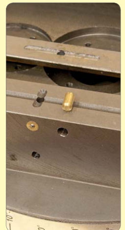
86. Showing the gib strip, adjusting screw and locking screw and locking lever brass dowel.
