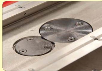
94. Lock retaining plate screws.
