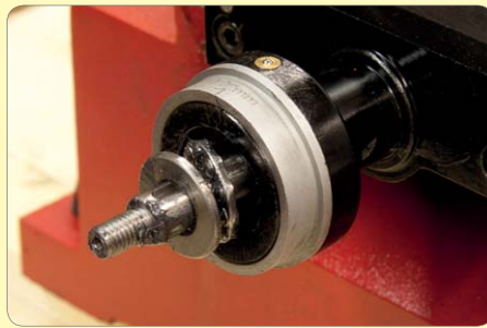
208. Grease & fit outer thrust bearing.
