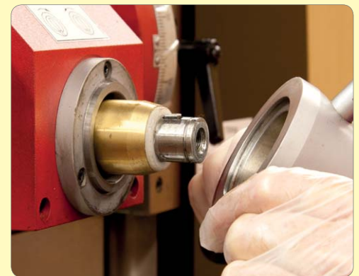
20. Remove handwheel assembly.
