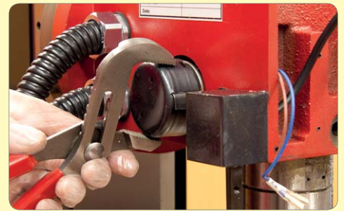
24. Carefully unlatch the spindle return spring housing and remove.
