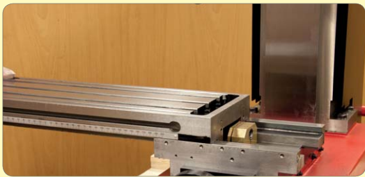
212. Oil table & saddle dovetails and slide the table onto the saddle.
