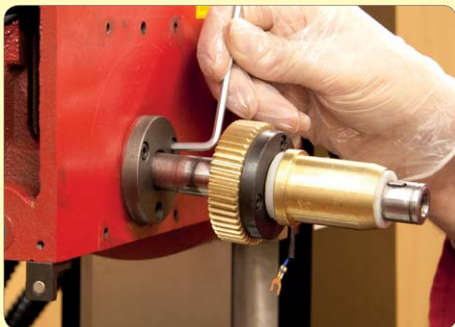
27. Remove 3 cap head screws from the flange and pull out the handwheel shaft.
