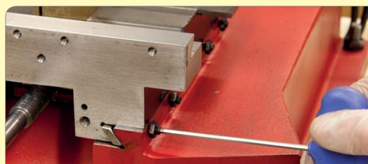
205. Lightly fit gib screws.
