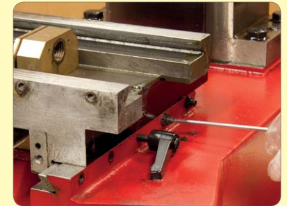
56. Remove gib screws & locking lever.
