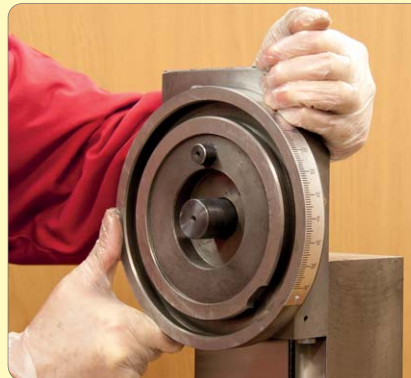
97. Slide onto column, rest on prop and tighten gib strip.
