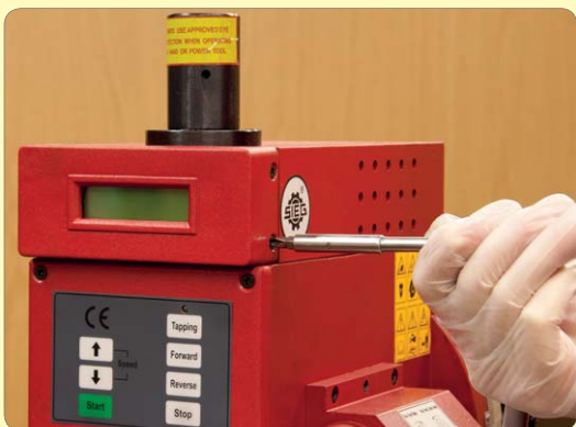
4. Remove the 6 screws securing the spindle speed display housing and pull away.
