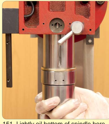
151. Lightly oil bottom of spindle bore, slide in spindle assembly and lock.
