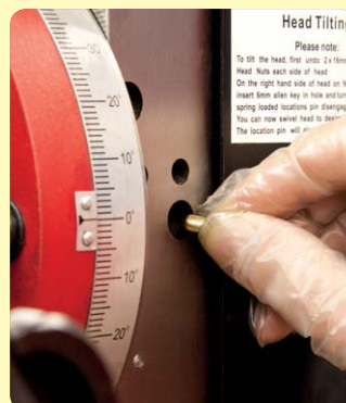
174. Fit brass plunger and locking lever.
