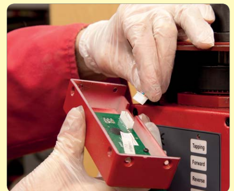
5. Unplug the speed display from the harness.
