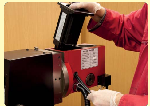
42. Lift out motor feeding wires through head.
