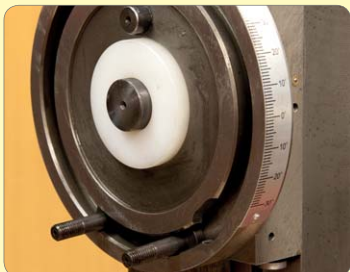
97. Fit plastic pressure disc with springs & fit T-bolts in T-slot.
