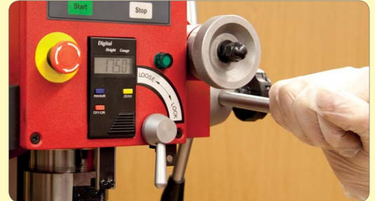
194. Work spindle up & down to check DRO operation.
