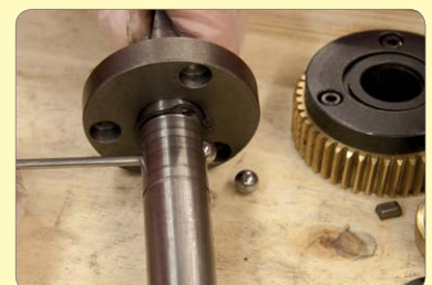
143. Push out 2 steel balls.
