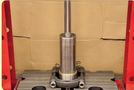
123. Press spindle out of sleeve.
