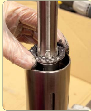
134. Grease and fit lower thrust washer, bearing and top thrust washer.
