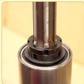
138. Fit lock nuts. Adjust and lock nut to preload.
