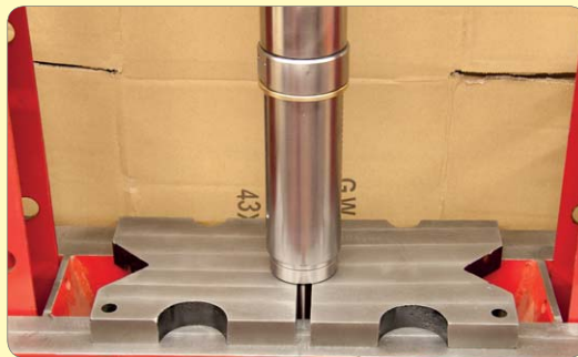
134. Grease and fit lower thrust washer, bearing and top thrust washer.
