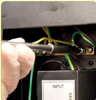
37. Disconnect motor earth wires.
