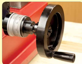
220. Fit handwheel assembly.
