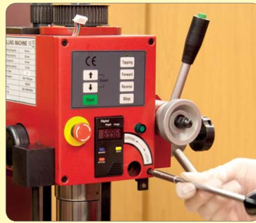
191. Fit control panel (checking no wires are trapped) and fix in place.
