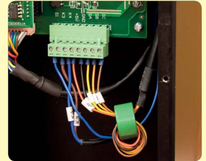
183. Wrap signal wires through ferrite core and connect to terminal block.
