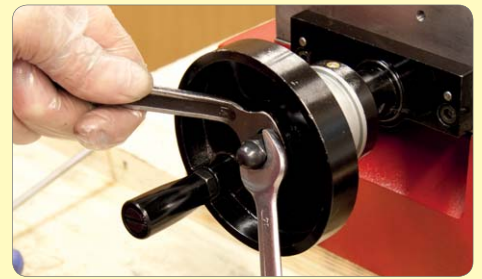
209. Fit key & handwheel assembly and adjust backlash.
