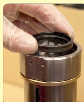
129. Fit inner grease shield.
