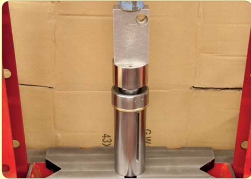
133. Press in spindle.
