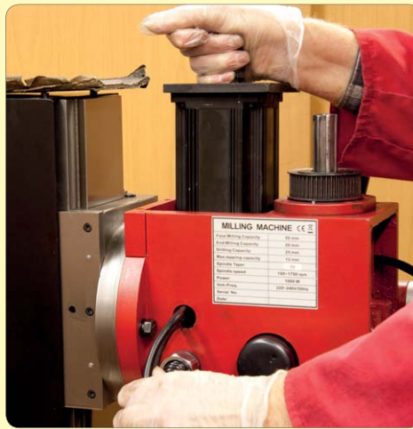
176. Lower motor into head whilst pulling cables out of side.
