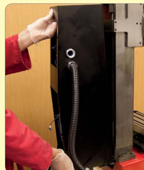
45. Remove rear panel assembly.
