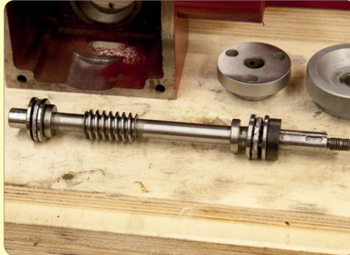
165. The worm shaft assembly.
