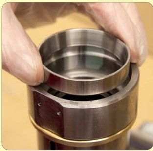
130. Fit and press in taper roller bearing outer race.
