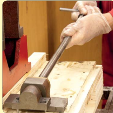
68. Unscrew leadscrew from nut pulling off the top bracket at the same time.
