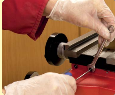
210. Final adjust gib screws for free movement/no slop in ways. Pinch up lock nuts.
