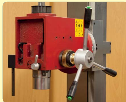
157. Position handwheel to your preference.
