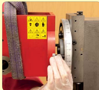
98. Offer head up and locate T-bolts through head.
