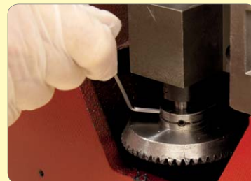
116. Adjust mesh on gears, lock screws and grease.
