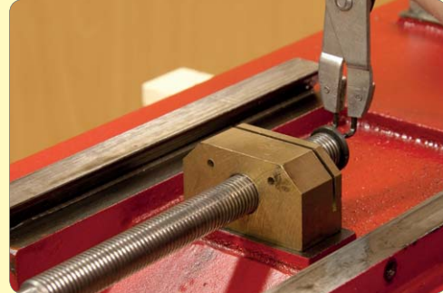
58. Remove circlip and washer.
