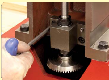
115. Fit X-axis screw assembly. Tap in taper pins & tighten bolts.
