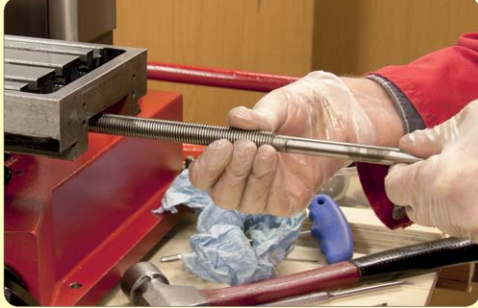
50. Remove X-Axis screw.
