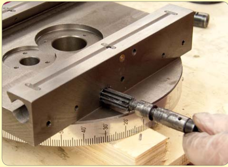
87. Grease and fit shaft into vertical slide.
