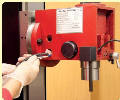
167. Fit rear electronics panel and feed cables through to front of head.
