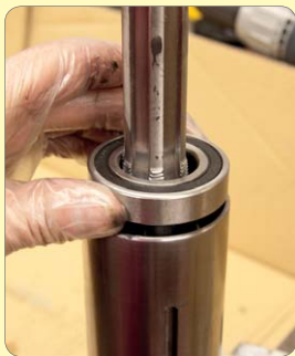
136. Fit and press in top bearing.
