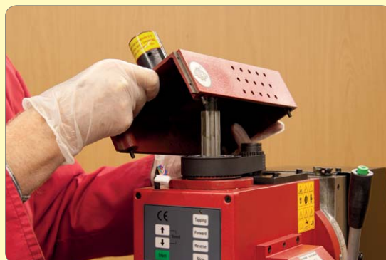
4. Remove the 6 screws securing the spindle speed display housing and pull away.
