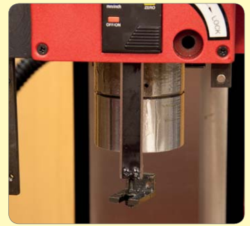
11. Pull down DRO bar level with spindle - DO NOT pull out.
