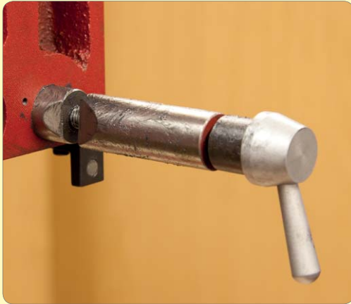
150. Assemble, grease and fit the spindle lock.
