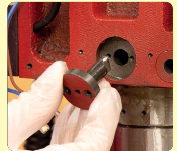
17. Undo 2 screws from spindle sleeve location dowel and remove.
