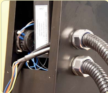
182. Fit lead tube to gland and feed wires to exit lower opening.
