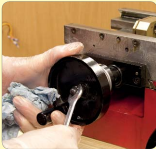
53. Remove Y-Axis Handwheel.
