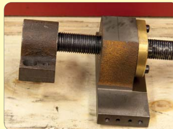
109. Press top bearing bracket onto Z-axis leadscrew.
