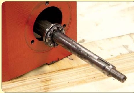
104. Fit inner thrust bearing assembly.
