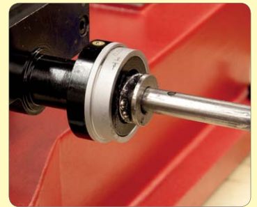
218. Grease & fit outer thrust bearing.
