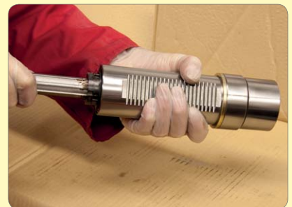
139. Check free movement of spindle.
