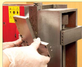
61. Undo 10 cap heads and remove both side plates.
