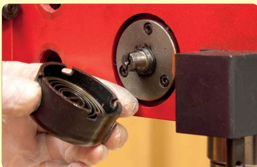
159. Fit the spindle spring return unit.
