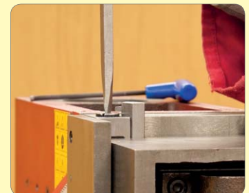
118. Tighten gib to lock head.
