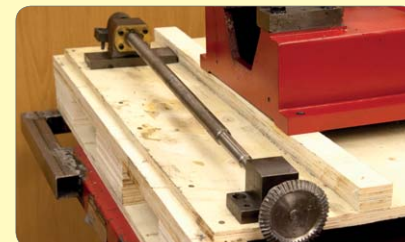
63. Undo Z-Axis lower bracket cap heads and lift out complete Z-Axis screw assembly.
