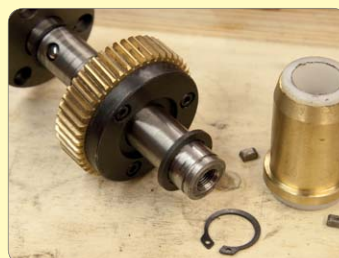
142. Slide off washer and gear.
