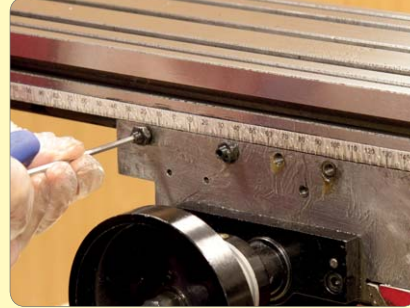
51. Remove gib screws & locking lever.
