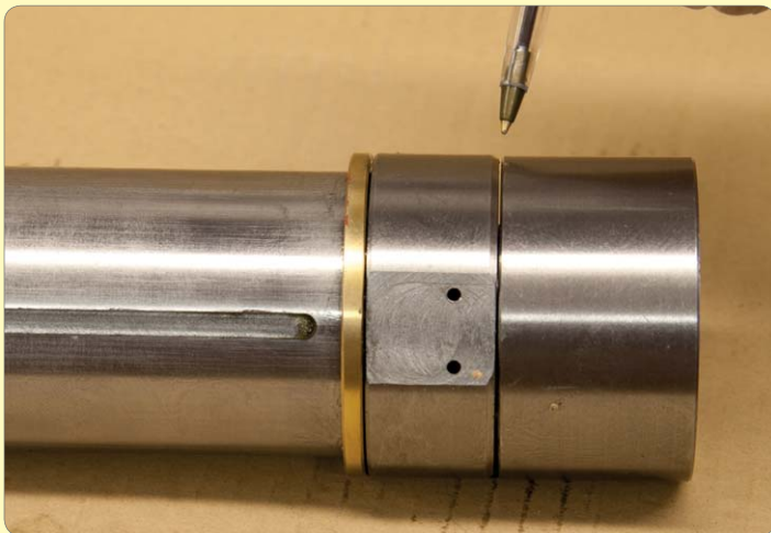
127. Suggested Modification: Reduce the diameter of the spindle flange to assist with any future dismantling.
