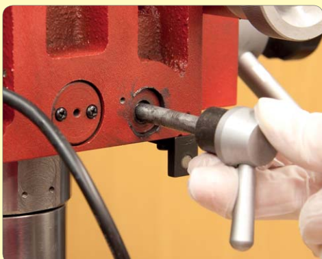
187. Temporarily remove the spindle sleeve lock.
