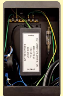
183. Wrap signal wires through ferrite core and connect to terminal block.
