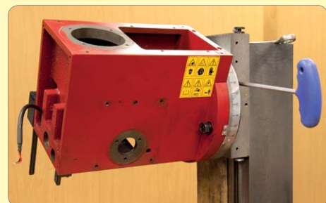
100. Using Allen key, disengage location shaft by turning clockwise, then spin head.
