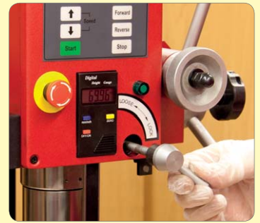
192. Re-fit the spindle sleeve lock.
