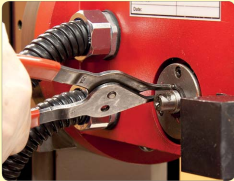
25. Remove the handwheel shaft retaining circlip.
