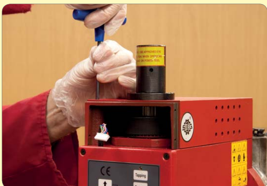
4. Remove the 6 screws securing the spindle speed display housing and pull away.
