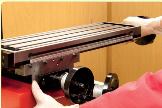
222. Wind table to one end & place thumb over the joint between saddle and base. Push & pull on table to check slop. Repeat this on joint between saddle and table. Adjust gibs if necessary to minimise any slop.
