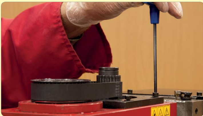
29. Remove motor plate fixing screws.
