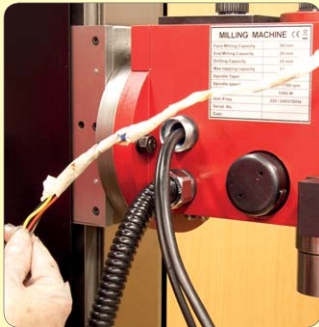
178. Tape up end of motor wires.
