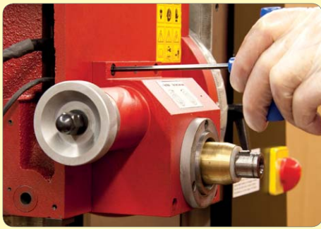
23. Undo the 4 screws securing the fine feed housing and lift housing away from the head.
