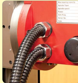
180. Fit lead tube to gland.
