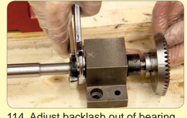
114. Adjust backlash out of bearing block and lock up.
