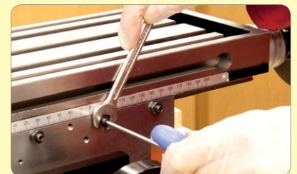
221. Final adjust gib screws for free movement/no slop in table. Pinch up lock nuts.
