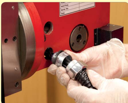
43. Undo and remove lower gland from head.
