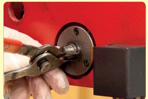
158. Fit retaining circlip.
