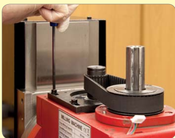
195. Fit belt & adjust tension.
