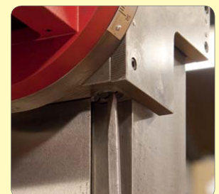
121. Slacken off gib screws. Wind head up and down and adjust gib to suit and tighten lock screw.
