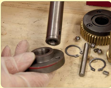
148. Slide off mounting flange.
