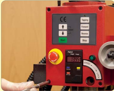
12. Remove the 4 screws securing the front cover assembly.
