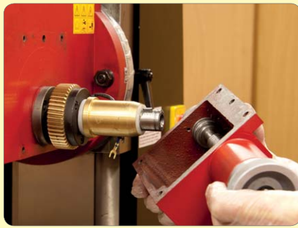
23. Undo the 4 screws securing the fine feed housing and lift housing away from the head.
