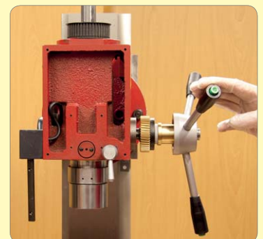
160. Check that spindle returns.
