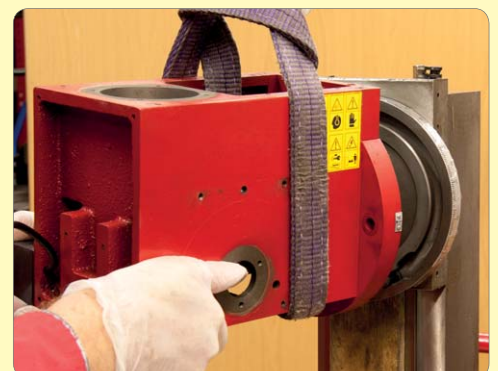
77. Pull head away from carrier bracket.
