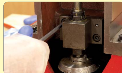
63. Undo Z-Axis lower bracket cap heads and lift out complete Z-Axis screw assembly.
