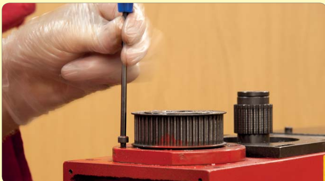
31. Undo 4 cap head screws and lift out the belt pulley housing.
