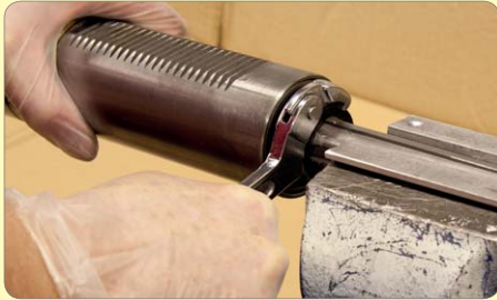
122. Undo and remove lock nuts & washer from spindle assembly.
