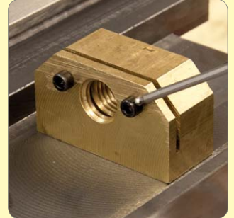
211. If necessary, adjust Y-axis backlash from rear of saddle.
