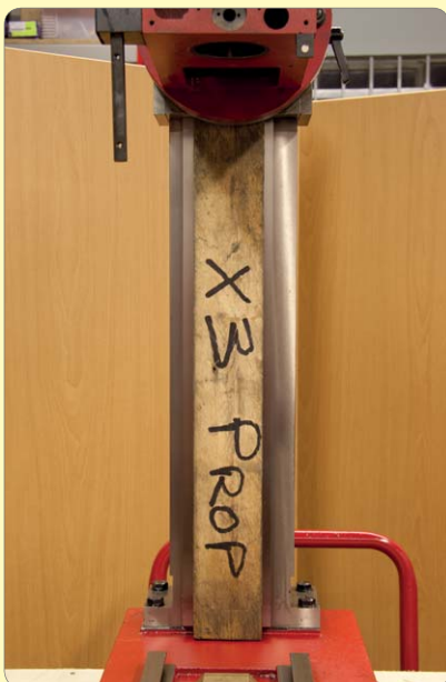
60. Wind head all the way to the top and prop in place.
