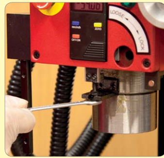
10. Slacken the locknut attaching the DRO bar to the bracket.
