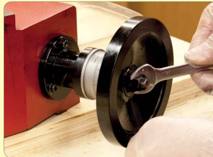
70. Remove Z-Axis handwheel.
