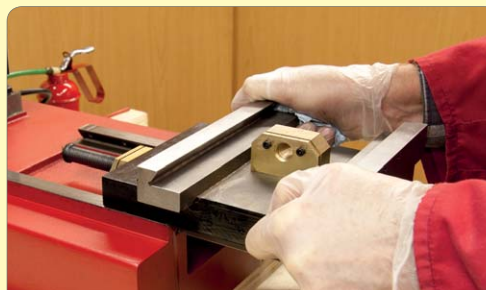
202. Oil bed and saddle dovetails and assemble.
