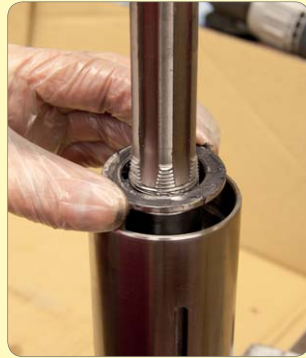
134. Grease and fit lower thrust washer, bearing and top thrust washer.
