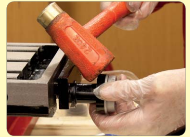
49. Undo cap heads & tap off bracket.
