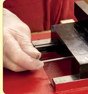
211. If necessary, adjust Y-axis backlash from rear of saddle.
