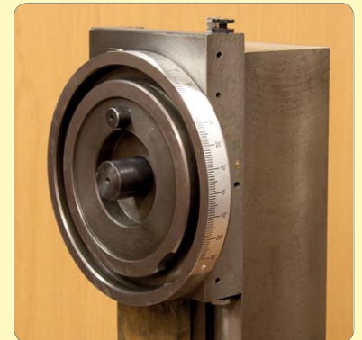
95. Grease and fit the gib adjusting and locking screws.
