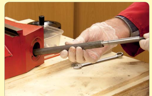
74. Pull out Z-Axis handwheel shaft.
