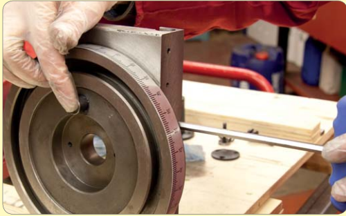
90. Engage splines & wind-in using Allen key.
