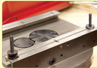
95. Grease and fit the gib adjusting and locking screws.
