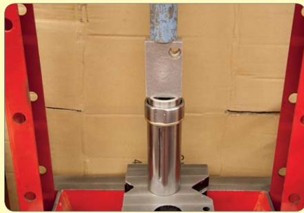
130. Fit and press in taper roller bearing outer race.
