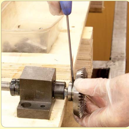
64. Undo 2 grub screws and remove gear.
