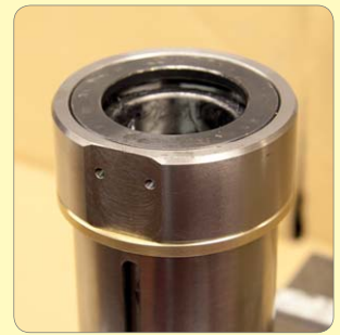
132. Fit outer grease shield.
