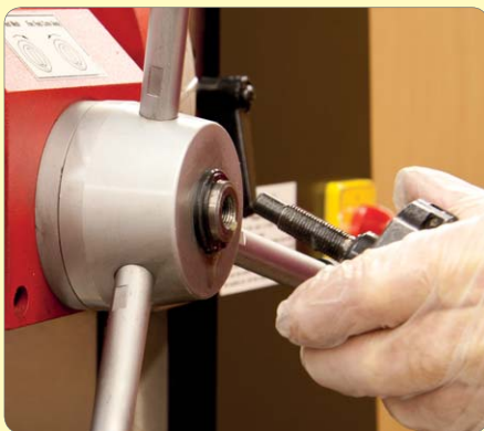
18. Remove the fine feed locking knob.
