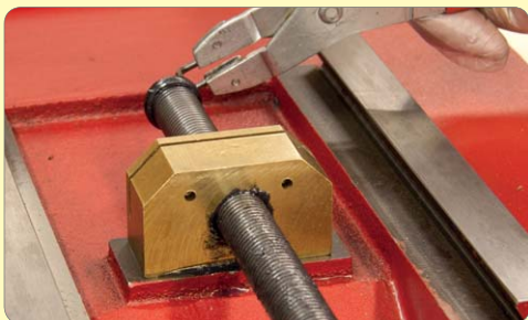
201. Grease/oil Y-axis screw and nut and assemble. Fit washer and circlip.
