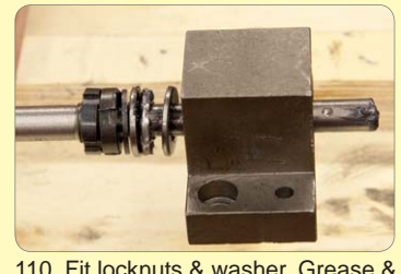
110. Fit locknuts & washer. Grease & fit upper thrust bearing & block.
