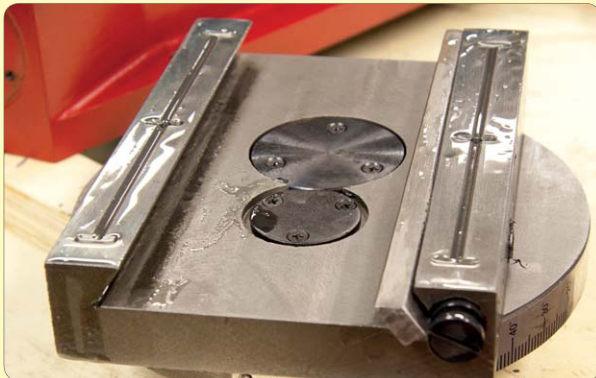
96. Locate gib strip slot on adjusting screw and oil dovetails.
