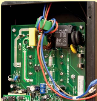
184. Wrap motor wires through ferrite core & connect to terminal block.
