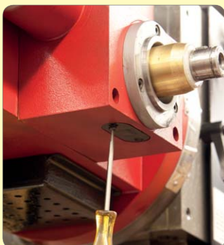
21. Undo 2 screws under handwheel housing & disconnect contact strip.
