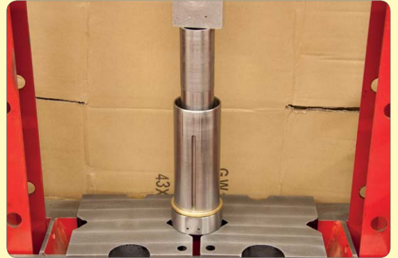
126. Press out the nose bearing & grease shields.
