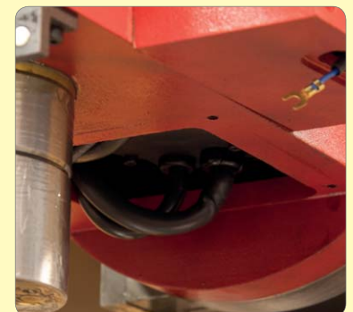
22. Undo 4 screws and remove wiring cover under head.
