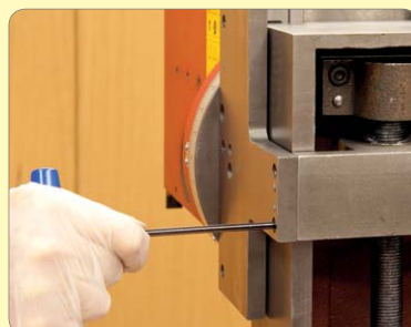
120. Lock side plate cap head screws.
