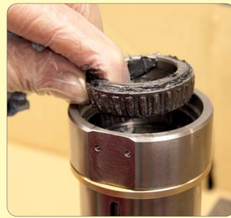
131. Grease and fit bearing.
