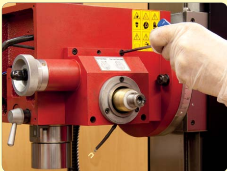
169. Fit fine feed housing to head.
