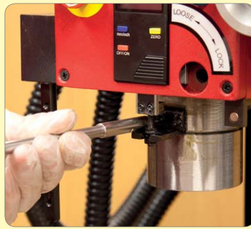
9. Unscrew the DRO Bracket from the spindle sleeve.
