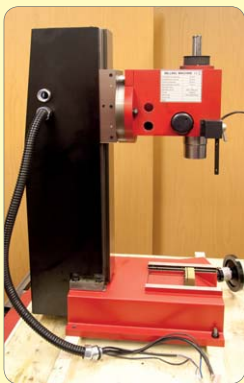
167. Fit rear electronics panel and feed cables through to front of head.
