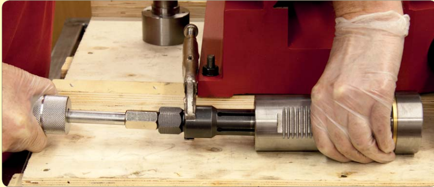
125. Use a bearing puller to remove the top bearing.
