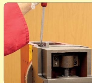
121. Slacken off gib screws. Wind head up and down and adjust gib to suit and tighten lock screw.
