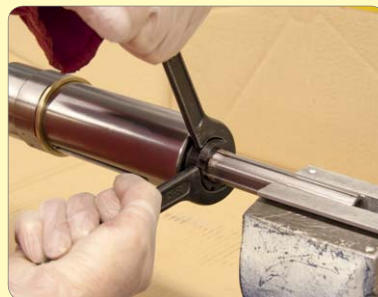
138. Fit lock nuts. Adjust and lock nut to preload.
