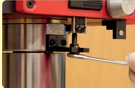
193. Attach the DRO bracket to the spindle sleeve and pinch the lock nuts up.
