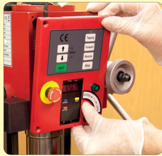
191. Fit control panel (checking no wires are trapped) and fix in place.
