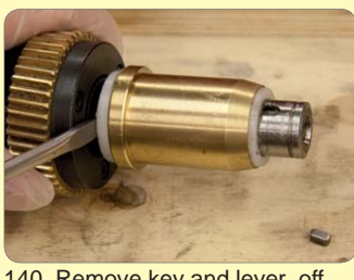
140. Remove key and lever off insulated bush assembly.
