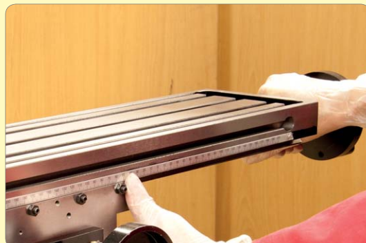
222. Wind table to one end & place thumb over the joint between saddle and base. Push & pull on table to check slop. Repeat this on joint between saddle and table. Adjust gibs if necessary to minimise any slop.
