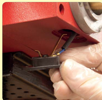
21. Undo 2 screws under handwheel housing & disconnect contact strip.
