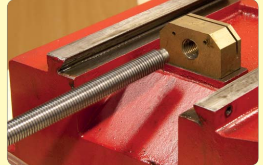
59. Remove Y-Axis screw.
