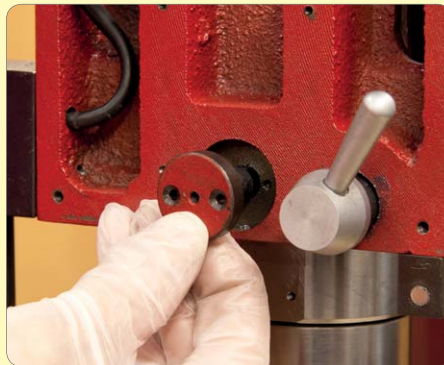
154. Grease and fit the spindle sleeve guide peg.
