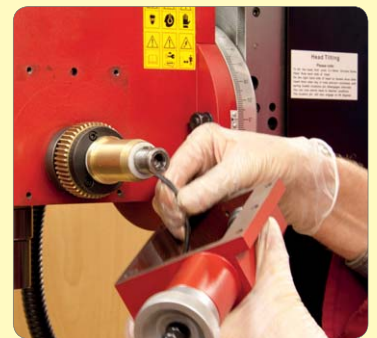
168. Feed cable through fine feed housing.
