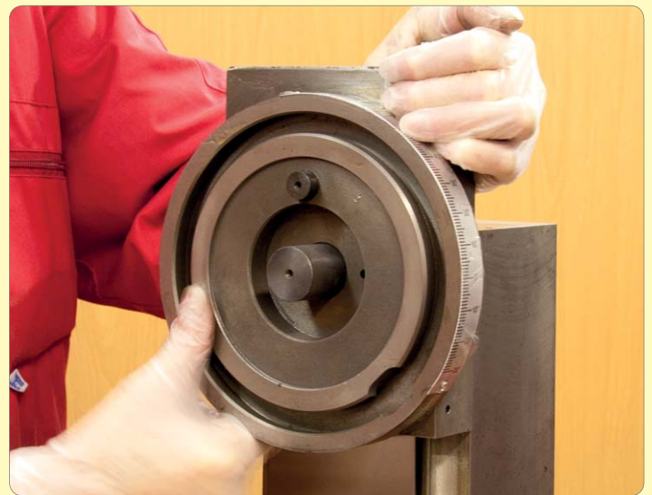
84. Lift off head carrier bracket / vertical slide assembly.
