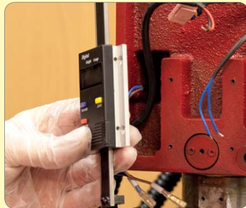
16. Undo 4 screws from DRO and remove from head.
