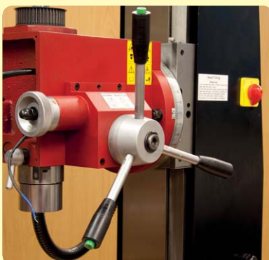
172. Fit key, handwheel, spacer & circlip.
