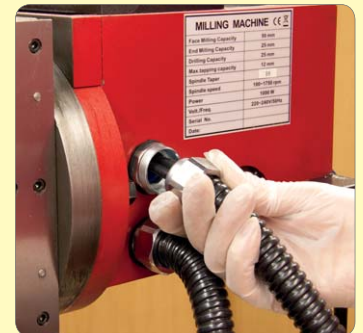
39. Undo gland nut at head end.
