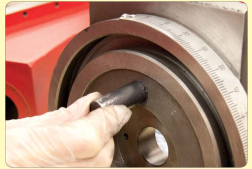
89. Grease and fit head location shaft.
