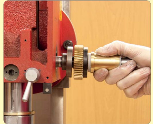
152. Grease and fit handwheel shaft assembly.
