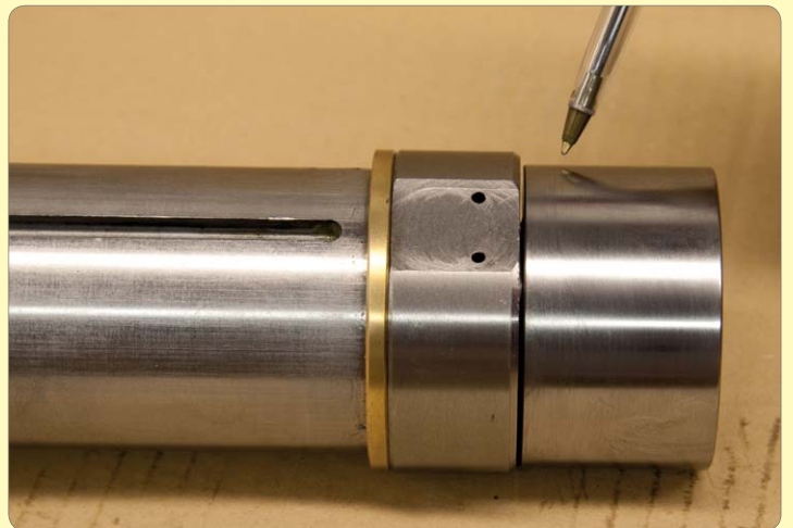
127. Suggested Modification: Reduce the diameter of the spindle flange to assist with any future dismantling.
