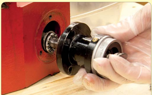
72. Remove 3 screws & pull off bearing assembly.
