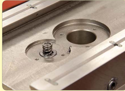
91. Fit spring in back of shaft.
