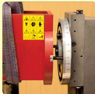
98. Offer head up and locate T-bolts through head.
