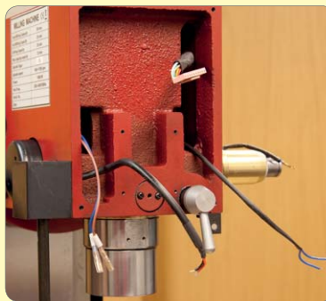
167. Fit rear electronics panel and feed cables through to front of head.
