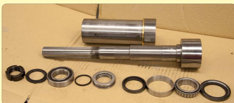
128. Spindle components laid out.
