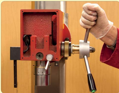
153. Temporarily fit the handwheel and wind up and down to check for free movement.
