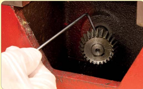
69. Undo 2 grub screws and remove gear.
