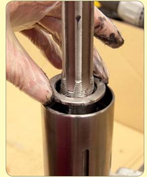
132. Fit outer grease shield.
