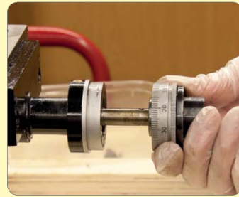
48. Pull off micrometer dial.
