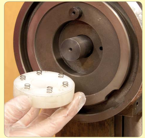
81. Pull off sprung pressure pad & springs.
