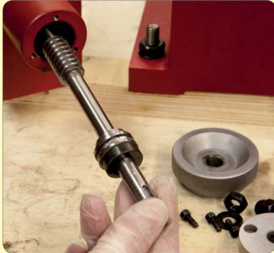
164. Remove the worm shaft.
