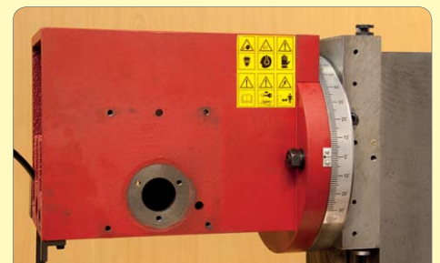
102. Return head to 0° and lock down nuts.
