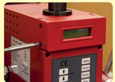
194. Work spindle up & down to check DRO operation.
