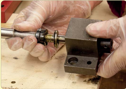
67. Remove bearing block assembly.
