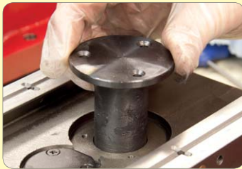
93. Fit head rotation spigot.
