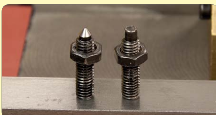
204. Modify gib screws to a cone point
