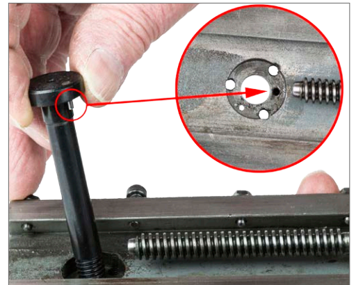
3. Insert the new stud into the compound slide ensuring the location pin enters the location hole.
