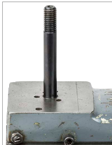
5. Attach the Model 000 Quick Change Tool Post onto the stud.
