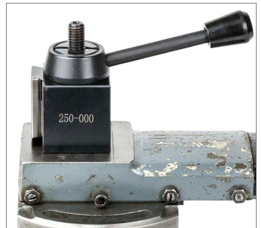
5. Attach the Model 000 Quick Change Tool Post onto the stud.
