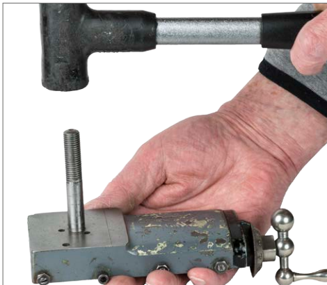
2. Remove the existing tool post stud, tapping with a mallet if necessary.
