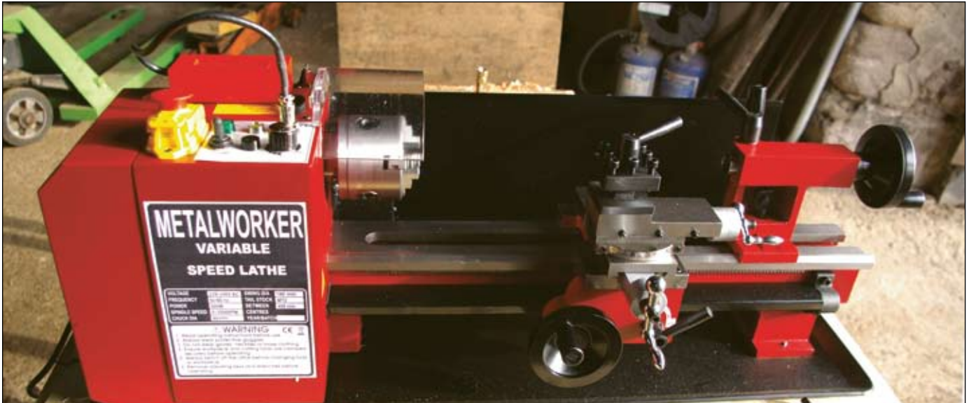
1. New Mini Lathe. The main visible changes are the control panel and leadscrew guard.
