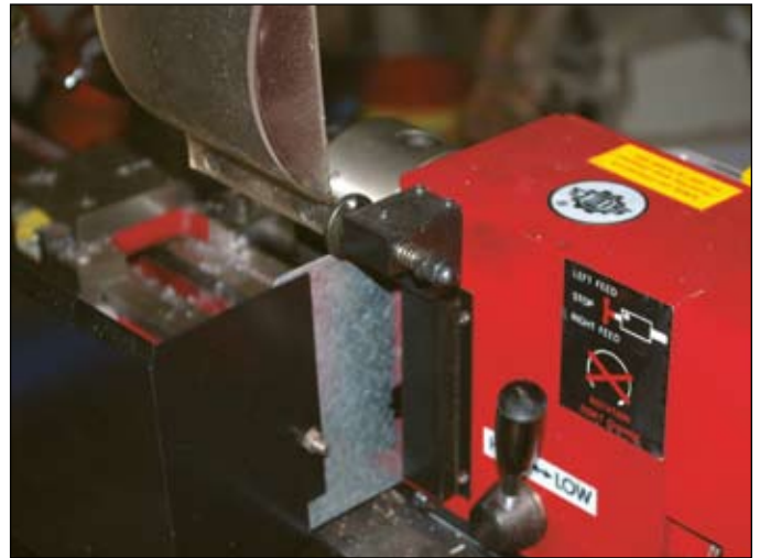
7. The older style chuck guard hinge and safety switch.
