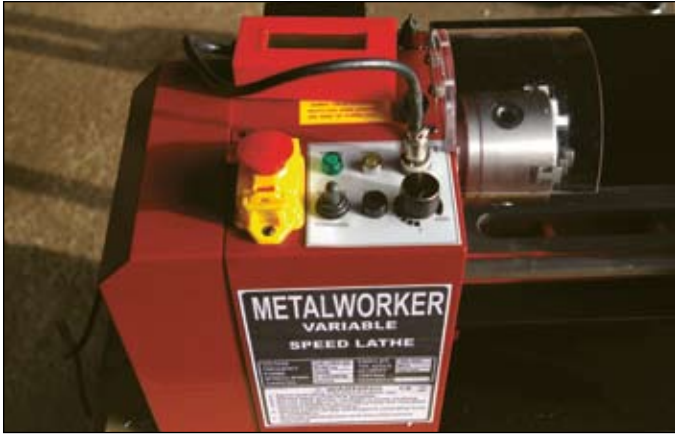
8. The new style control panel with add on speed read out.
