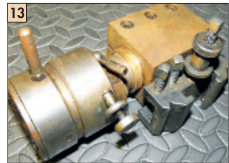
13 A Coventry diehead with a Dickson type holder, a possible future project?
