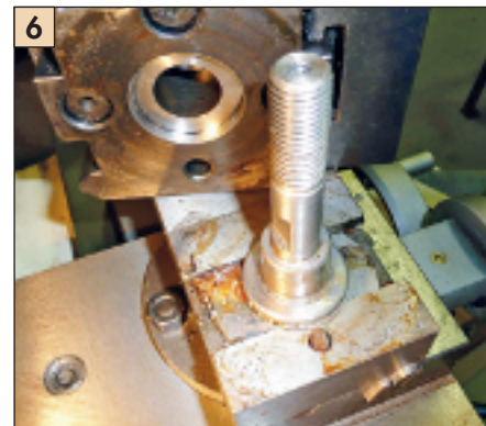
The Dickson style QCTP requires a stepped mounting post.
