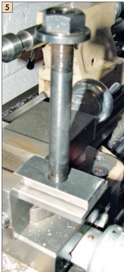
The top of the mounting plate is just below the top slide surface.
