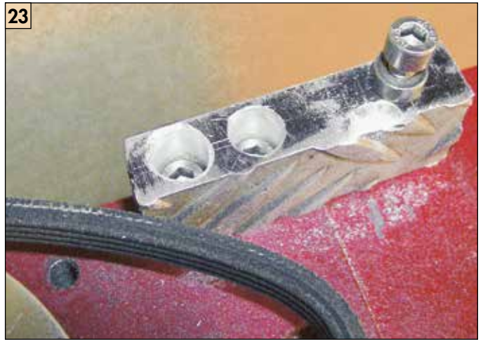
23 Counterbored holes in a spacer and fixing screw washers.
