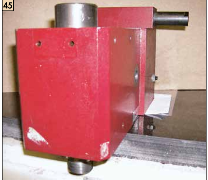
Using a surface plate to true up the milling head.
