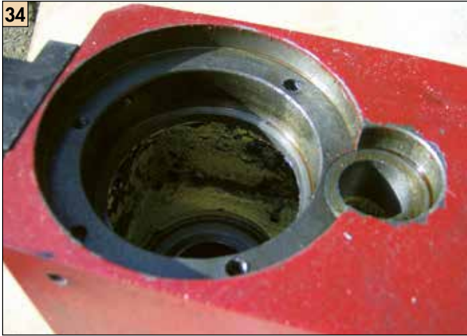
34 The spindle came free with the bottom bearing.
