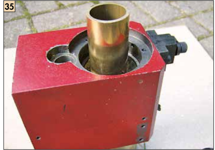
35 Using a brass drift to extract the top bearing.
