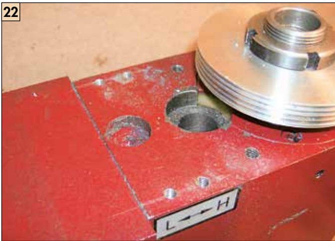
22 Four tapped holes need to be made in the head for the spacers.
