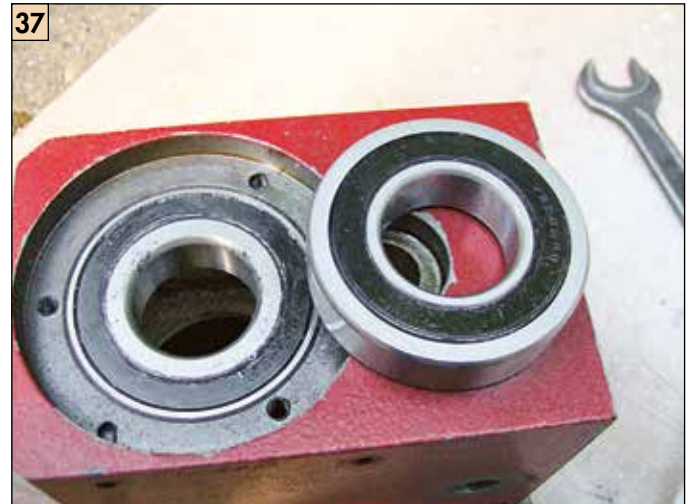
37 Comparing the two sides of the angular contact bearings.
