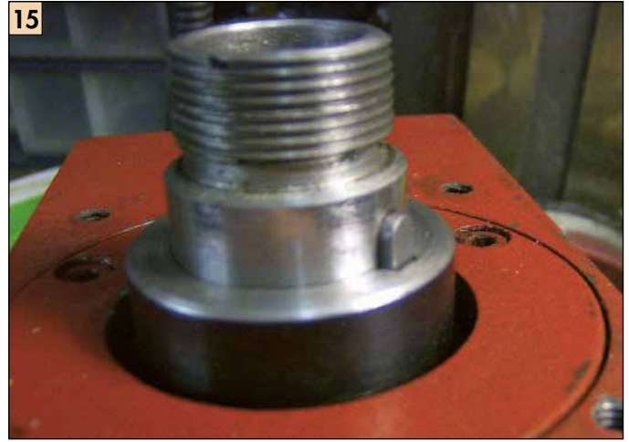
15 The shortened spacer leaves room to fit the pulley.
