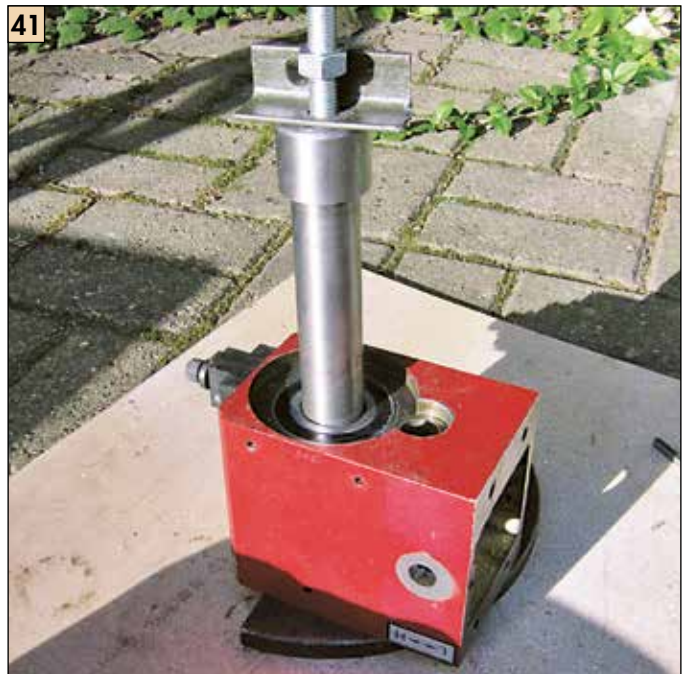
41 The set-up to start drawing in the spindle.
