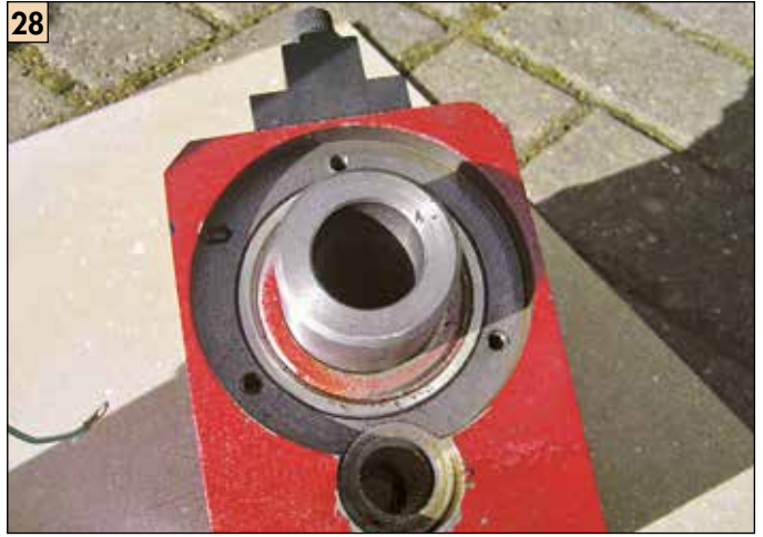
28 The lower end of the spindle with the bearing cover removed.
