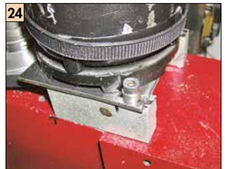
24 The clamp bolts and spacers hold the motor in place.
