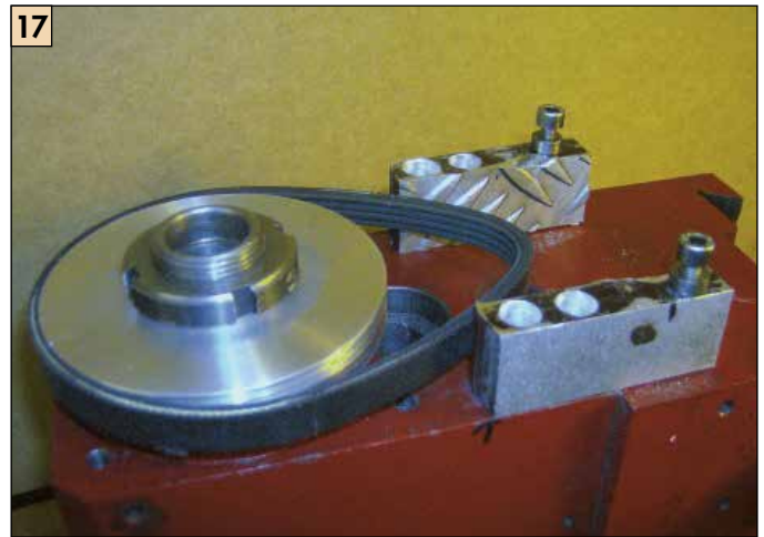
17 This photo shows how the ring nut clamps the pulley to the spindle.
