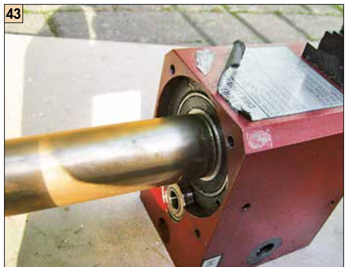
43 A stout tube allows the spindle to pass through the top bearing.
