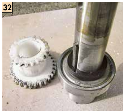
32 The spindle and the final drive gear. The keyway on the spacer is misaligned.
