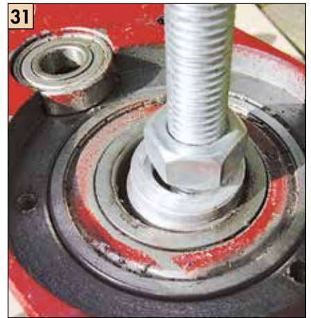
31 The spindle immediately after it has come free of the top bearing.
