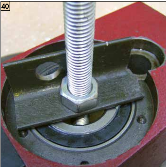
40 The bottom bearing fully home.
