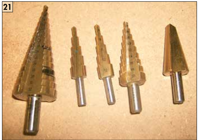
21 A series of step drills and a cone drill.
