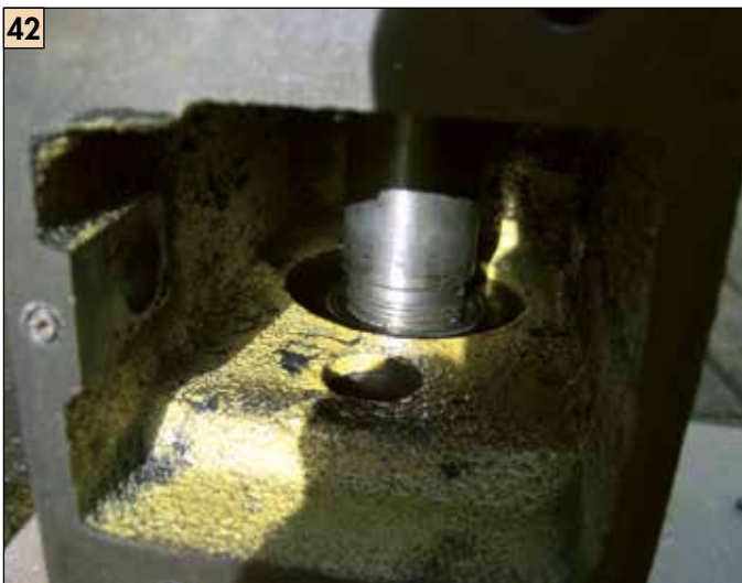
42 The spindle starting to enter the top bearing.
