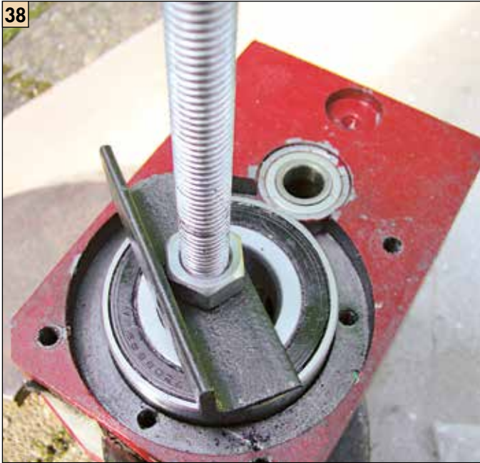
38 Drawing in the top bearing.
