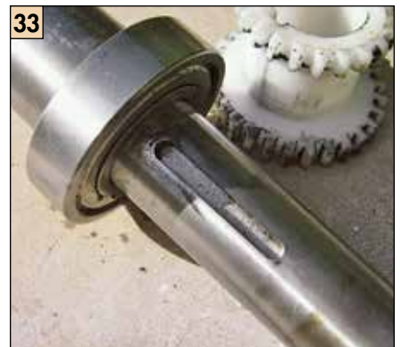
33 The keyway after removal of the spacer.
