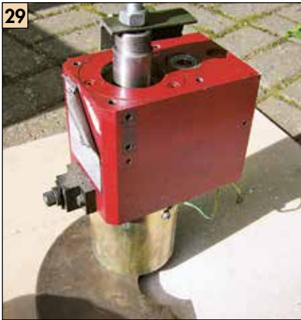
29 The initial setup for drawing the spindle.
