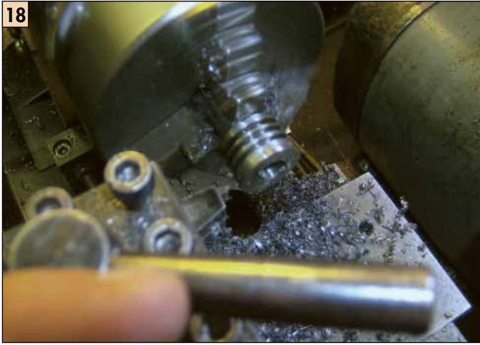
18 About to cut the fourth groove in the small pulley.
