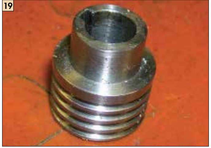
19 The small pulley is just 19mm in diameter.
