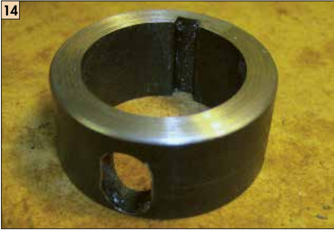
14 The spacer above the top bearing must be reduced at both ends if the belt drive conversion is made.
