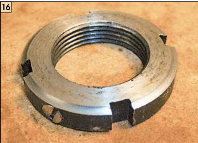
16 The ring nut used to apply bearing preload.
