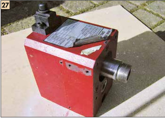
27 The spindle housing, note the bearing cover.
