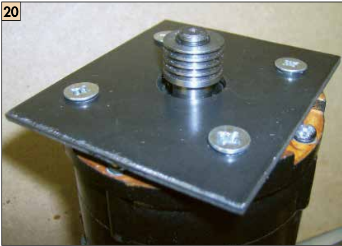
20 The motor plate and small pulley before cutting the fixing slots.
