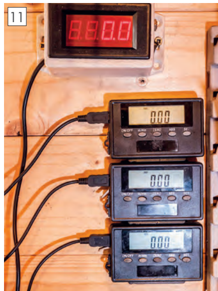
11 Remote read out heads for the scales.
