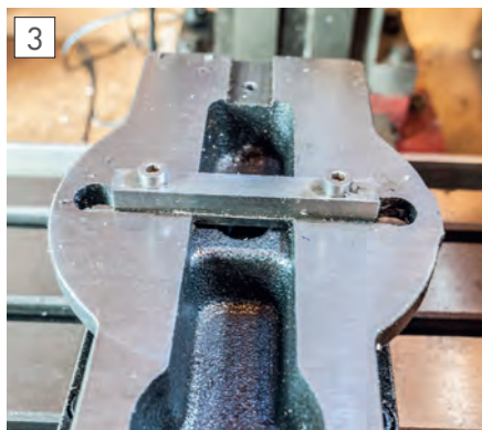
Underside of modified machine vice.
