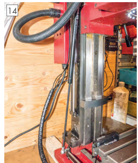
Gas strut in position and fully extended.
