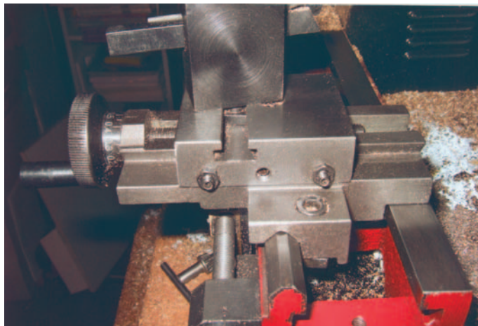
Saddle, cross slide and lathe bed. The front 'Shear' takes the form of an inverted 'V', the back one is oblong in profile. The cross slide adjusting screws and toolpost fixing 'Tee Slot' are clearly shown.
