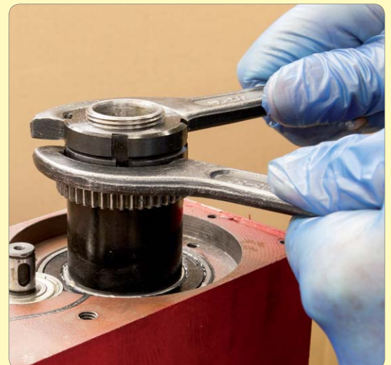
21. Fit lock nuts, set bearing preload and lock the nuts.
