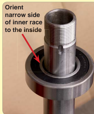
11. Fit 7206B angular contact bearing noting orientation.
