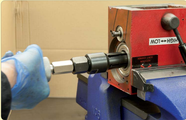
9. Drift out rear bearing.
