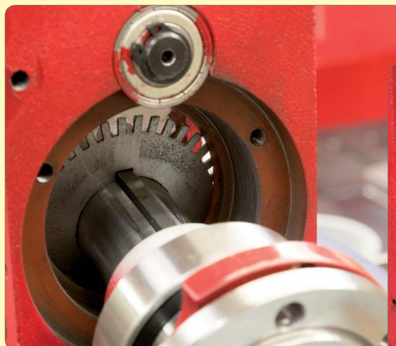
14. Align keyway in speed readout disc, spacer and gear and push spindle home.
