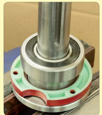
12. Press bearing onto spindle.
