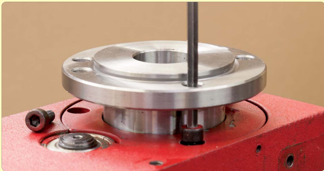
24. Lock front bearing cover in place.
