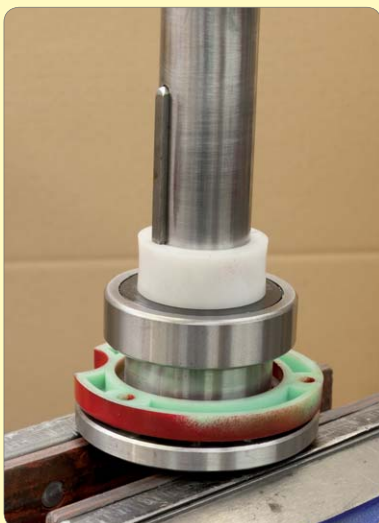
13. Fit small spacer and key.
