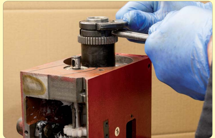
2. Remove the lock nuts from the spindle.
