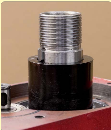
19. Fit black metal spacer and key.
