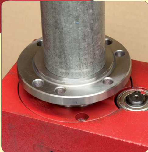
15. Final press spindle assembly into head.
