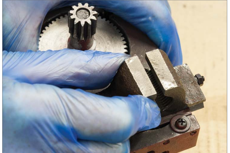
16. Check there is no slop in the half nuts.
