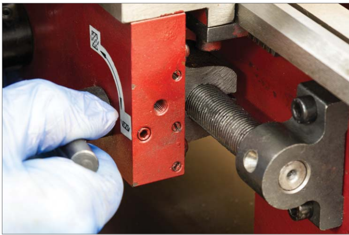
21. Lock the half nuts onto the leadscrew near the end of the bed.
