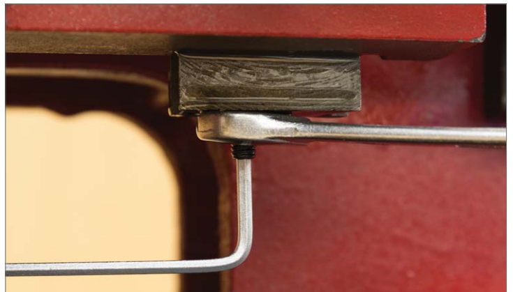
24. Lightly tighten the lower half nut adjusting screw and then back-off \frac{1}{4} turn. Lock the adjusting screw with the lock nut.
