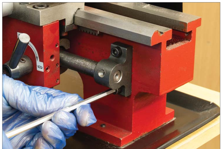
20. Re-fit the lead screw bracket with the screws finger tight.
