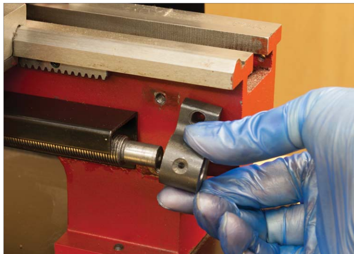
3. Remove the right hand leadscrew bracket.
