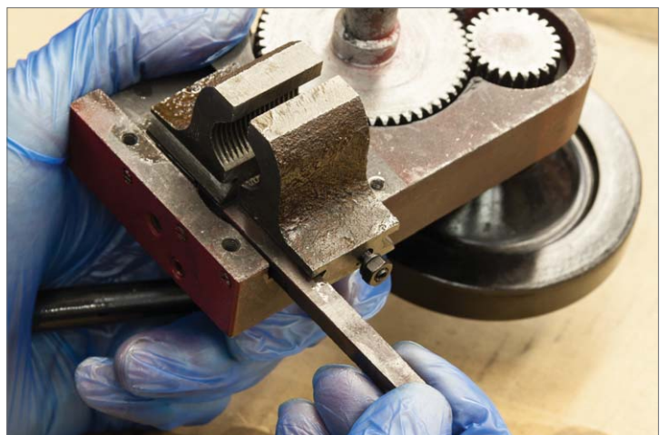
12. Lubricate the dovetail slide, locate the half nut pins in the slots of the cam disc and slide in the gib.
