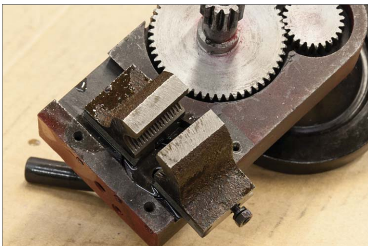
12. Lubricate the dovetail slide, locate the half nut pins in the slots of the cam disc and slide in the gib.
