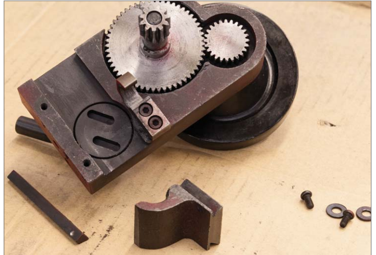
9. Remove the gib and half nut.
