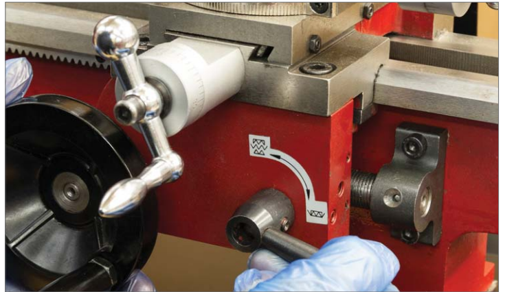
24. Check the bite of the half nuts and if necessary slacken and re-pin the apron screws. If everything is correctly aligned, finally tighten the apron screws and the leadscrew bracket screws.
