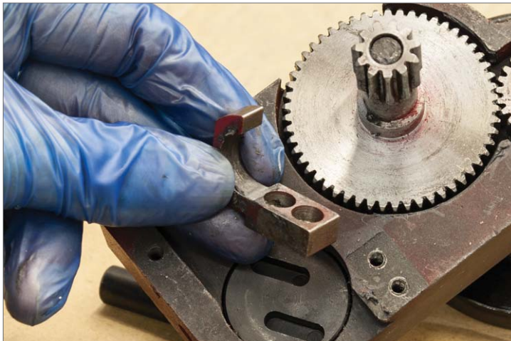
10. Remove the leadscrew support arm.
