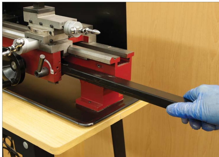
4. Slide out the leadscrew cover.
