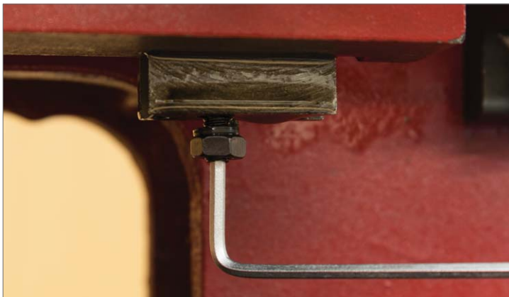
24. Lightly tighten the lower half nut adjusting screw and then back-off \frac{1}{4} turn. Lock the adjusting screw with the lock nut.
