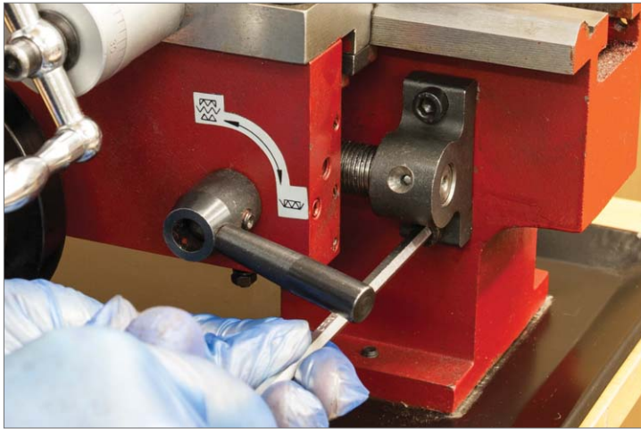
23. Slacken and then pinch the leadscrew bracket screws.
