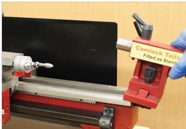
1. Remove the tailstock from the bed (as you can probably tell, this is a display model!).
