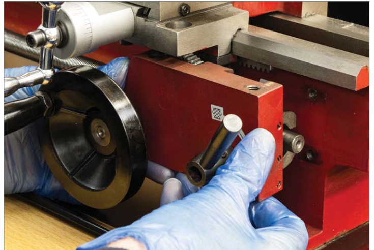
18. Slide the apron back into position.
