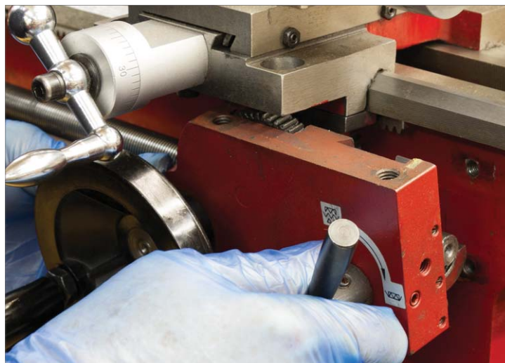
5. Remove the 2 hex socket head screws that fix the apron to the saddle and carefully slide the apron off the end of the leadscrew.
