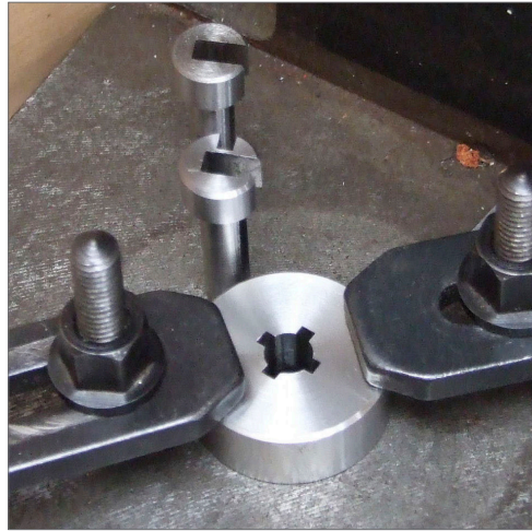
Fig 8. The finished item with 4 keyways
