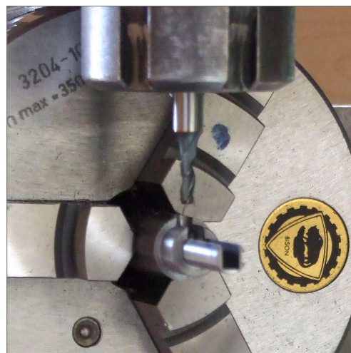
Fig 5. Machining the Broach slot 90 degrees to the shallow 2 mm keyway
