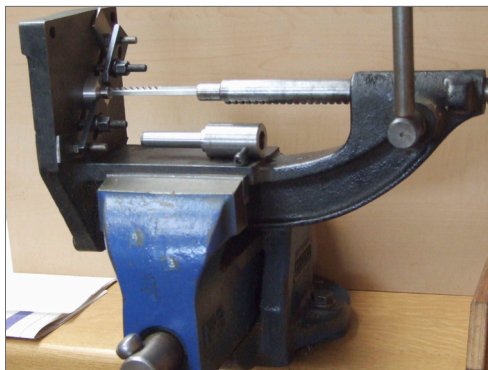
Fig 1. Cutting the first keyway
