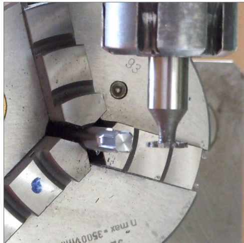
Fig 9. Milling the mating part using a 1.5mm wide Woodruff cutter
