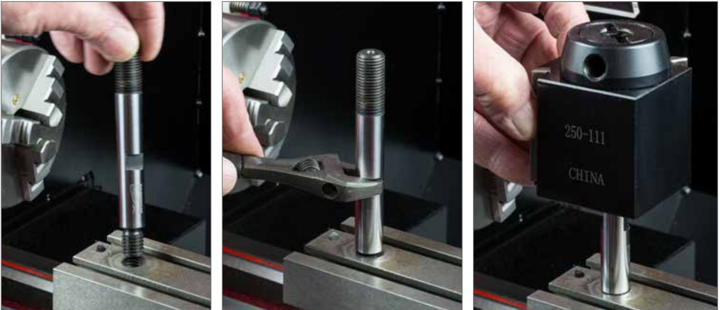
2. Screw the new tool post stud into the compound slide and tighten with a spanner.
