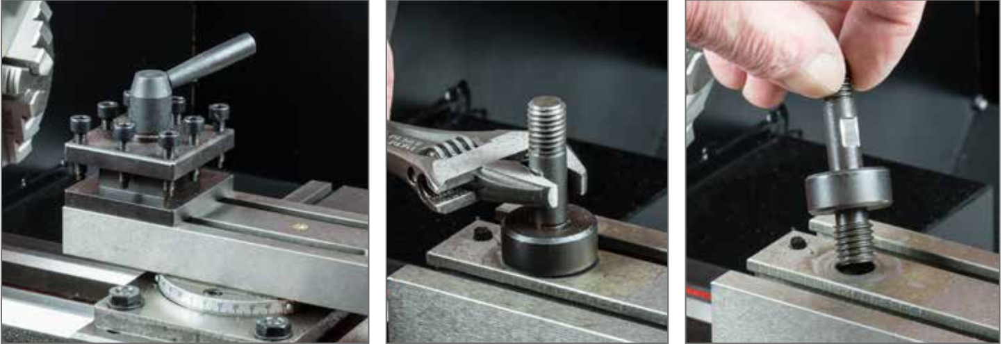
1. Remove the existing tool post and tool post stud from the compound slide.
