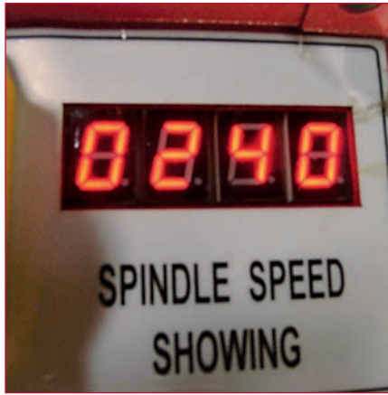
4 The tachometer shows the spindle speed.
