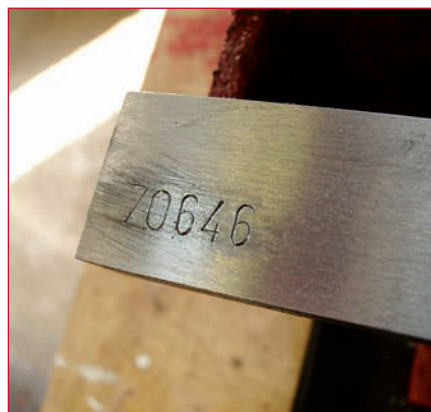
14 Raised metal around stamped numbers has been dressed off with lap.
