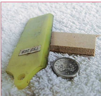
13 The diamond lap has been carved away at an angle to permit access to the root of the dovetails.
