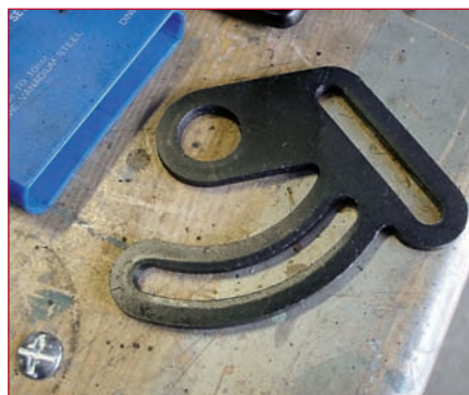
20 The tumbler bracket is a pressing with sharp edges on one face.
