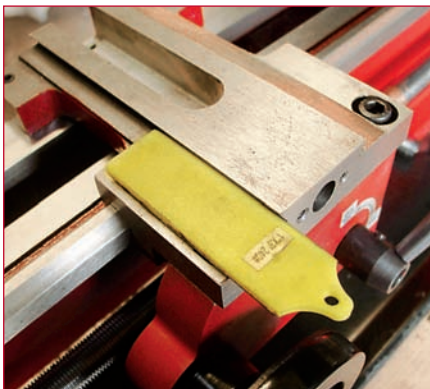
18 Milled surface of the cross slide dovetail is lightly rubbed with the lap.
