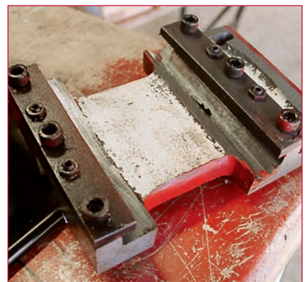
15 Underside view of saddle shows "push - pull" adjustment screws.
