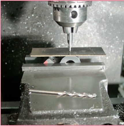
16 The RH leadscrew bearing being set up for drilling an oil way.
