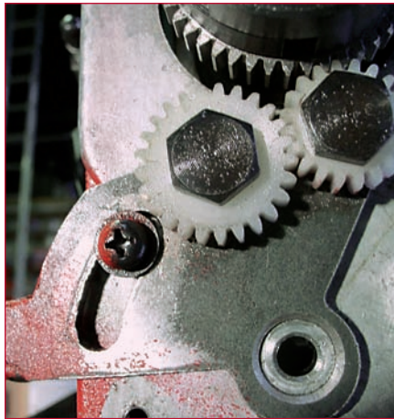
11 Showing clearance between larger white gear and washer.
