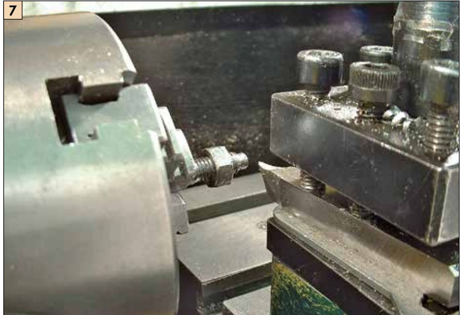
Cutting a 1mm pitch test thread.
