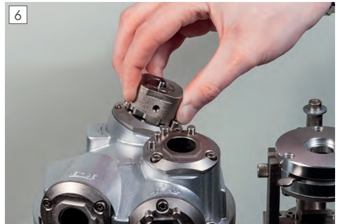
6 Putting on the secondary clearance.
