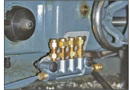
7. Multi-way manifold on the lathe carriage.
