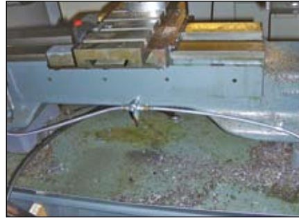
6. The three way connector on the back of the lathe bed.
