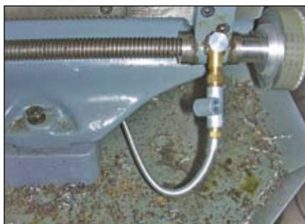
16. Tailstock end leadscrew bearing banjo.
