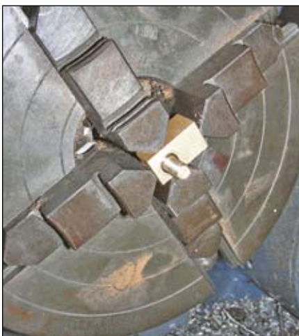
8. Turning and threading the connector.
