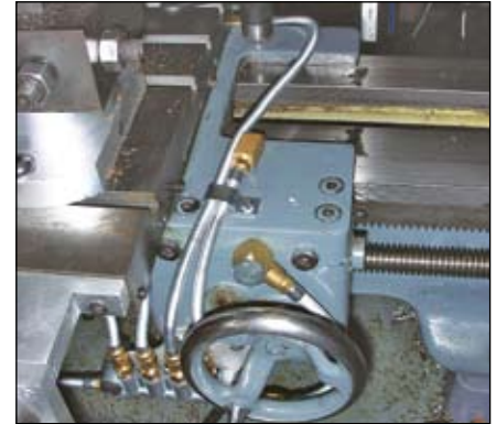
20. A final view of the carriage connections.
