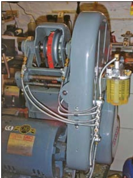
1. Most of the lubrication system can be seen in this photo.
