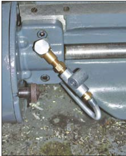
12. Banjo connector to leadscrew bearing.
