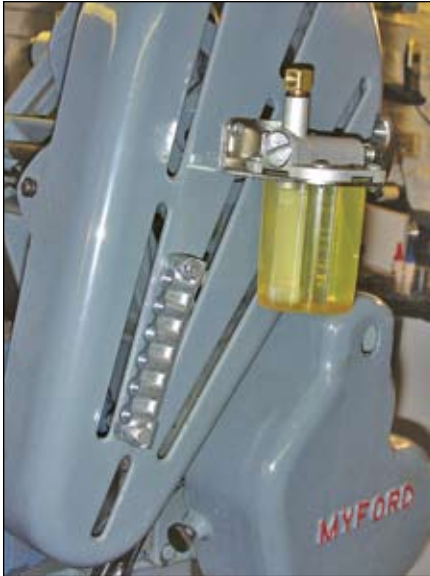
5. The reservoir is mounted on the belt guard.
